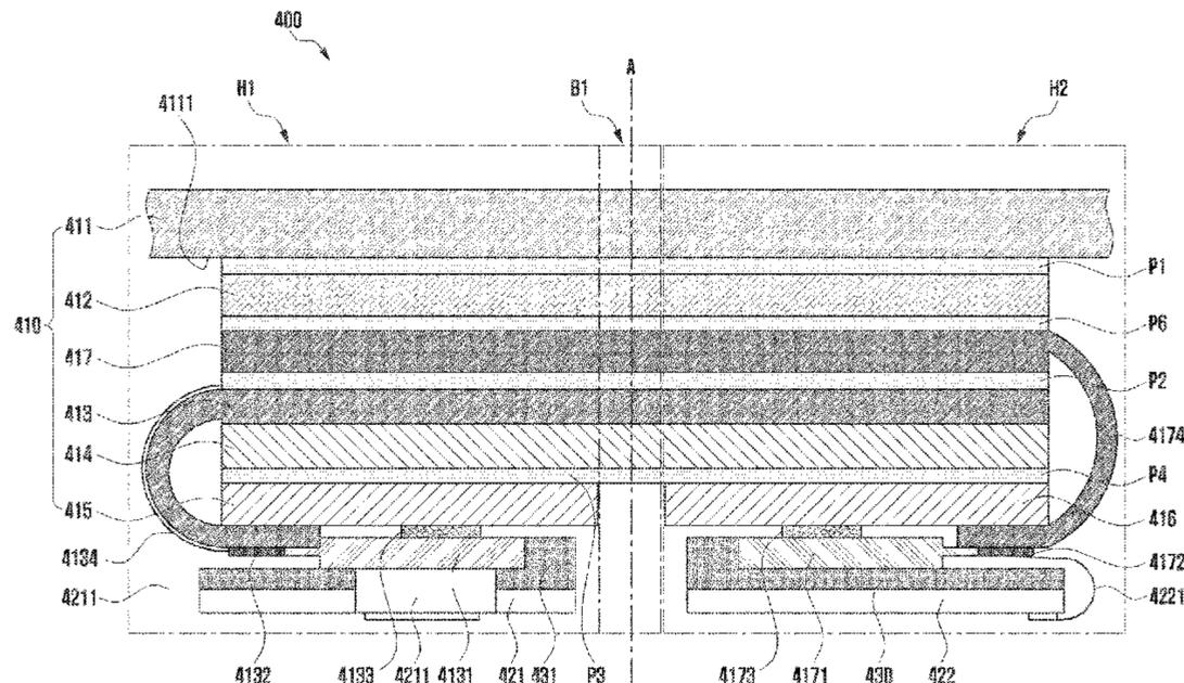
housing. The electronic device further includes a supporting member disposed between the second conductive member and the second PCB in the second housing. The second conductive member is electrically connected to the second PCB through a conductive region of the supporting member and electrically connected to the ground of the first PCB through the wiring member.
