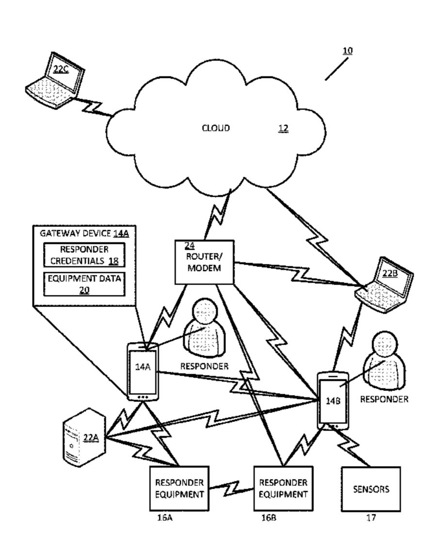
the translated equipment data to be relayed to a computer. The processor is also configured to register equipment data in the memory. The gateway device also includes a transceiver configured to receive the equipment data from external equipment, transmit responder credentials to the computer and transmit the translated equipment data to the computer.
