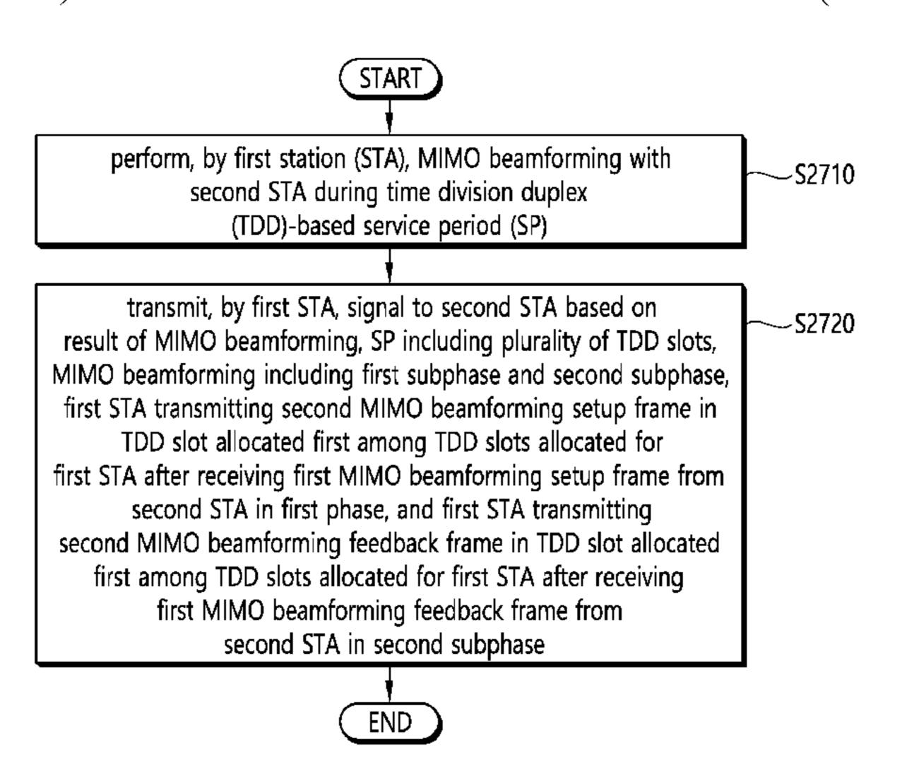
beamforming setup frame in the first allocated TDD slot among the TDD slots allocated to the first STA. In the second sub-step, after receiving a first MIMO beamforming feedback frame from the second STA, the first STA transmits a second MIMO beamforming feedback frame in a first allocated TDD slot among the TDD slots allocated to the first STA.
