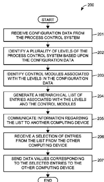
based upon the configuration data. The method includes generating a hierarchical list of available process data, and selecting from the hierarchical list a set of information to include on a watch list or alarm list.
