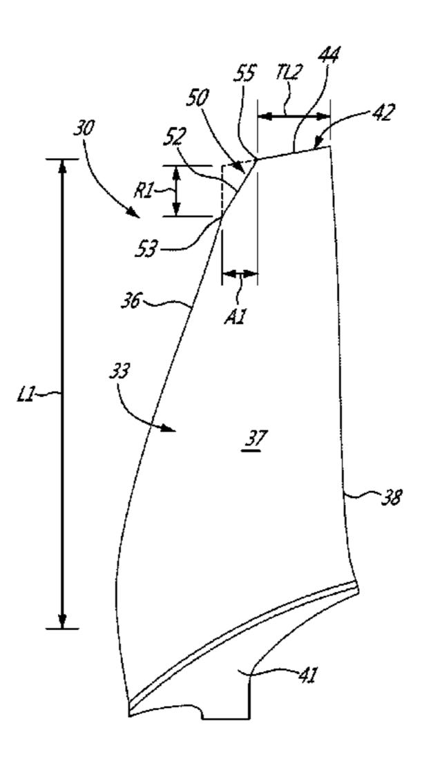
different blade types having means for generating different shock patterns between adjacent ones of the two or more different blade types when the gas turbine compressor operates in supersonic flow regimes. The means for generating different shock patterns on the modified blade aerodynamically mistune the two or more different blade types.
