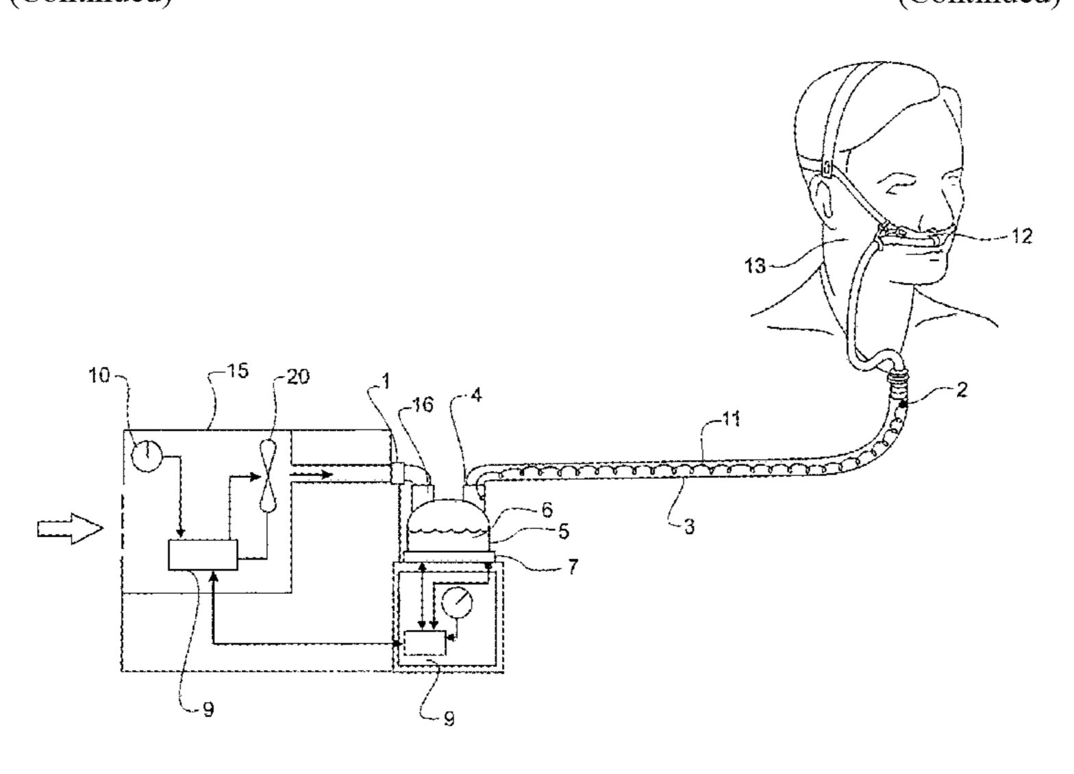
data relating to the sensed parameter from the RFID tag in real time, and adjusting the output parameters of the breathing circuit accordingly.
