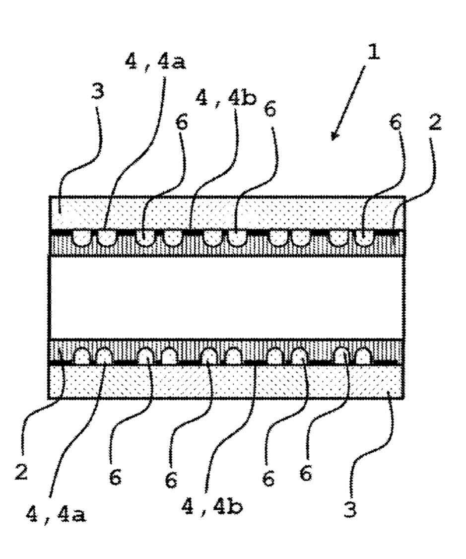
between the layers 2, 3 and 4, which allows forces to be transmitted from one of the layers 2, 3, 4 to another in a particularly reliable and permanent manner, as a result of which undesired delamination is prevented, in particular in flexible endoscope shafts 1.
