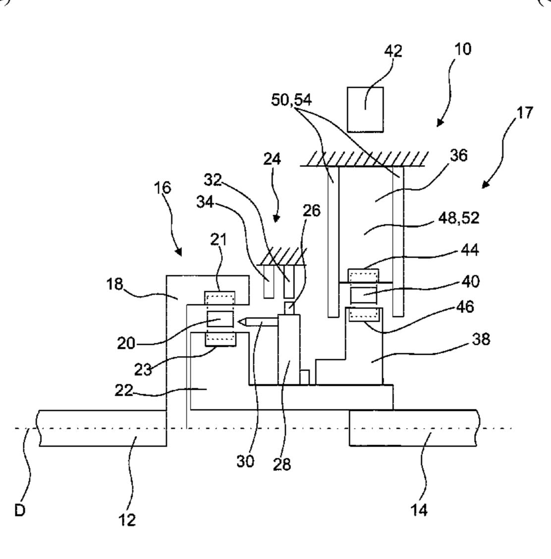
or vice versa. A holding plate is located adjacent to the at least one permanent magnet to suppress magnetic flux from the at least one permanent magnet to the brake unit. A motor vehicle drivetrain containing at least one clutch assembly is also provided.
