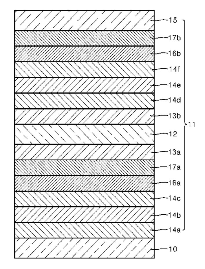
tric layer and the refractive index of the sixth dielectric layer are each lower than the refractive index of the fifth dielectric layer.
