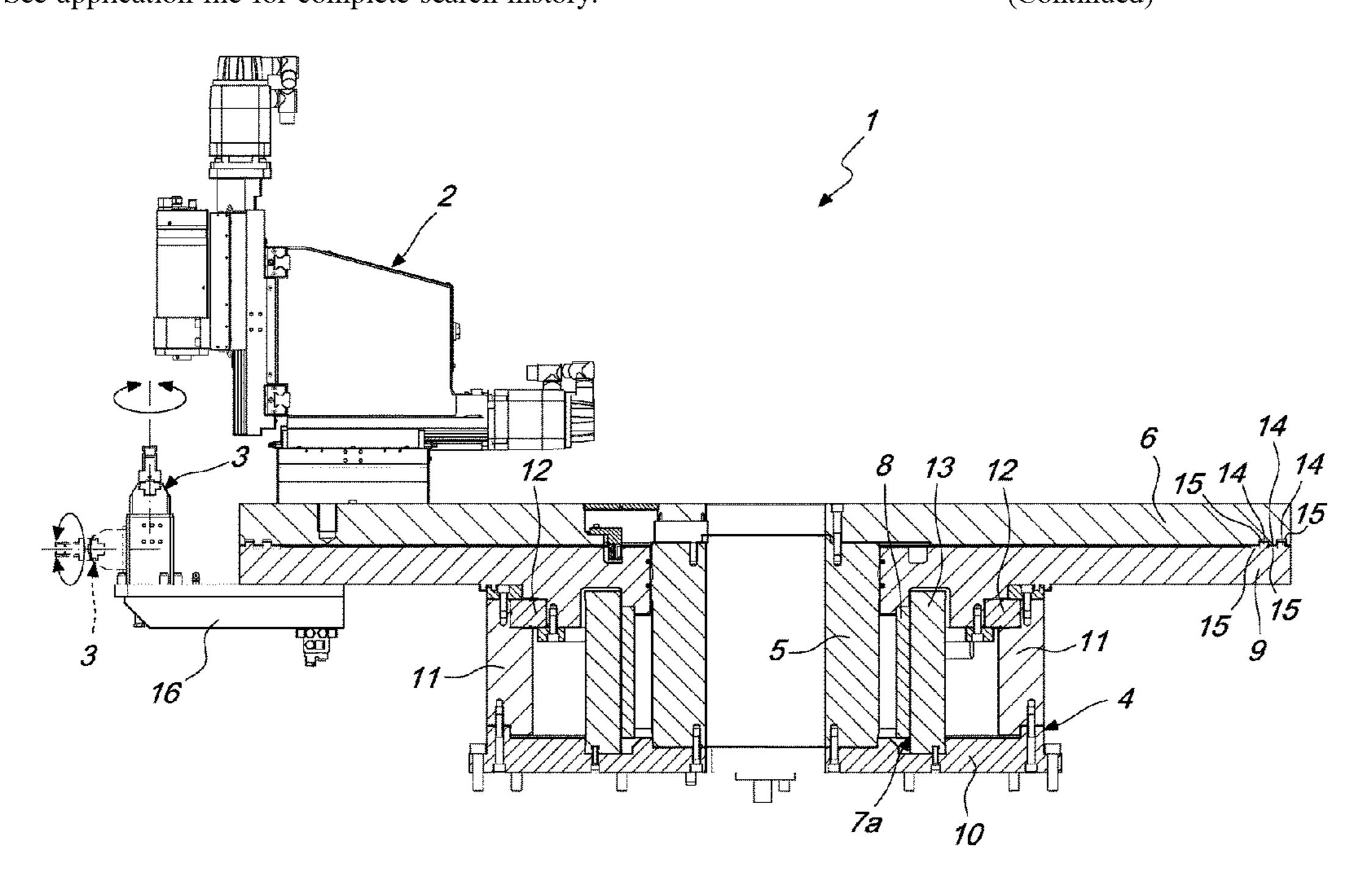
The center has a fixed footing, which is provided with a substantially central post for supporting a supporting surface for supporting the at least one machining station, a motor drive unit being coupled to the post.
