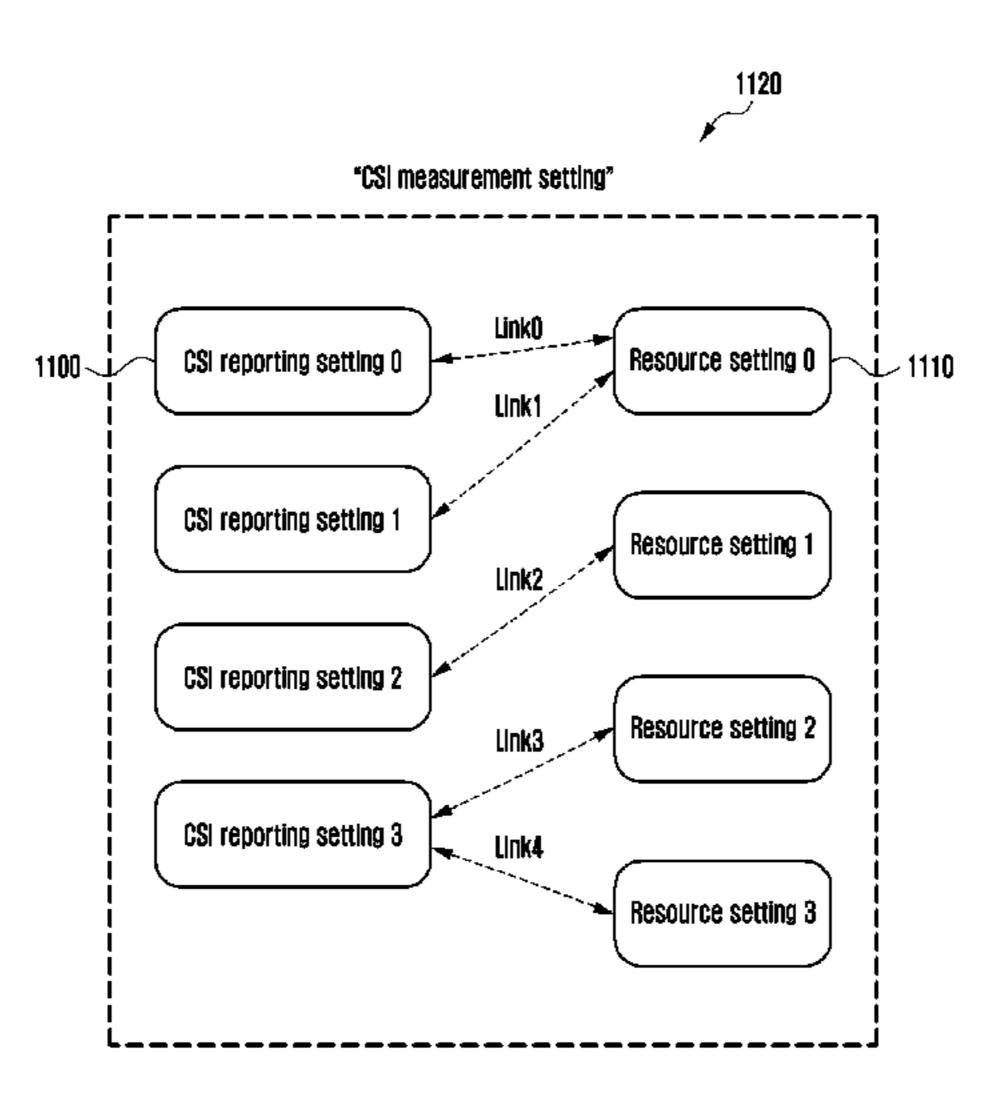
of the CSI-RS ports of the at least one CSI-RS resource within the resource set is 1 or 2, and the at least one CSI-RS resource within the resource set is regarded to be transmitted in different OFDM symbols, in case that the repetition information is set as on; and transmitting CSI based on the configuration for the resource set.
