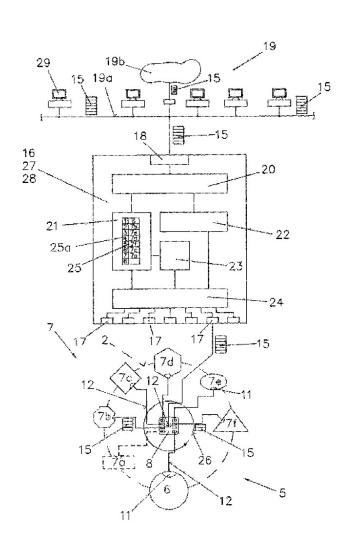
exchange with the company-internal network, e.g., an intranet and/or an internet, and with the production resources of the work cell, and establishes direct communication between the production resources. A software update can be performed in the work cell controller during the operation of the work cell. Furthermore, the work cell controller creates a list and assigns addresses for the connected production resources.
