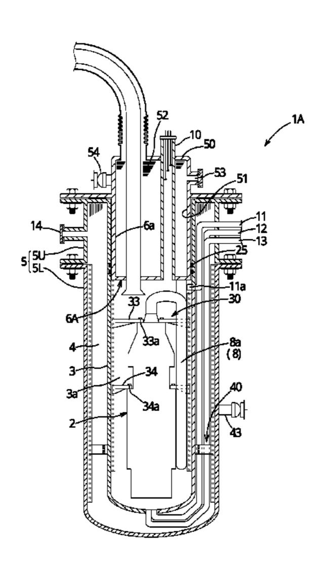
flange to upper ends of the inner and outer tanks upper part to a second flange to an outer circumferential part of the lid structure, and a second fastener to fasten with bolts, a third flange to an upper end of the outer tank body to a fourth flange to a lower end of the outer tank upper part. A vacuum insulating layer is formed between the inner and outer tanks.
