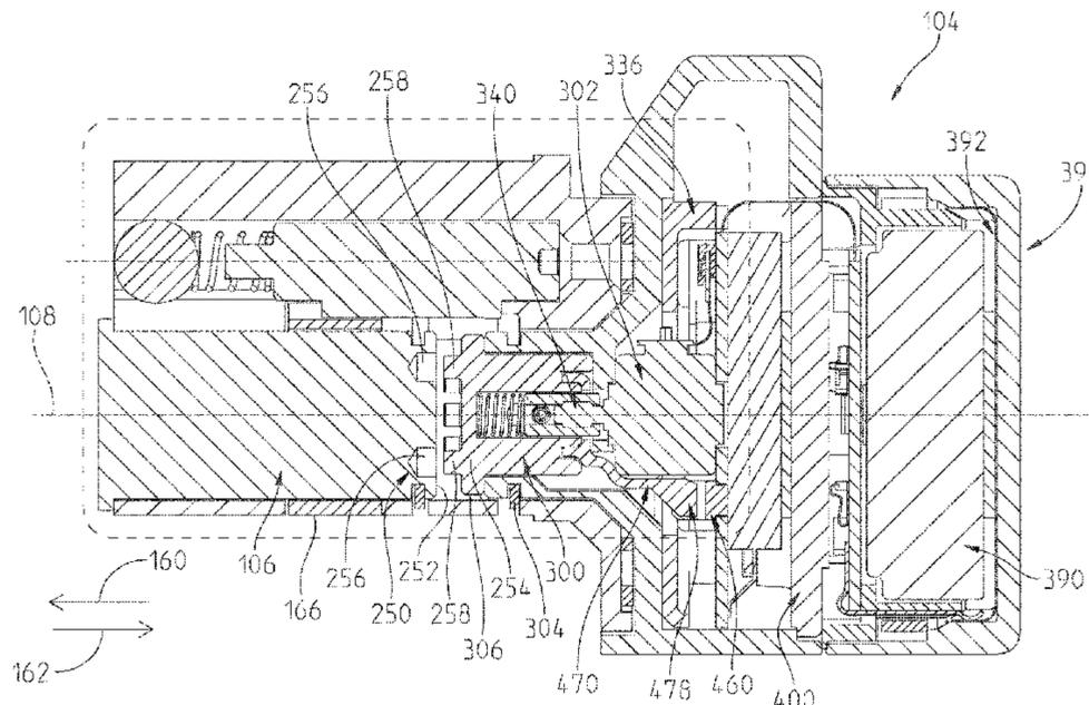
be positionable in a retain position wherein the core keeper extends beyond an envelope of lock core body to hold the lock core body in an opening of the lock device and a remove position wherein the core keeper is retracted relative to retain position to permit removal.
