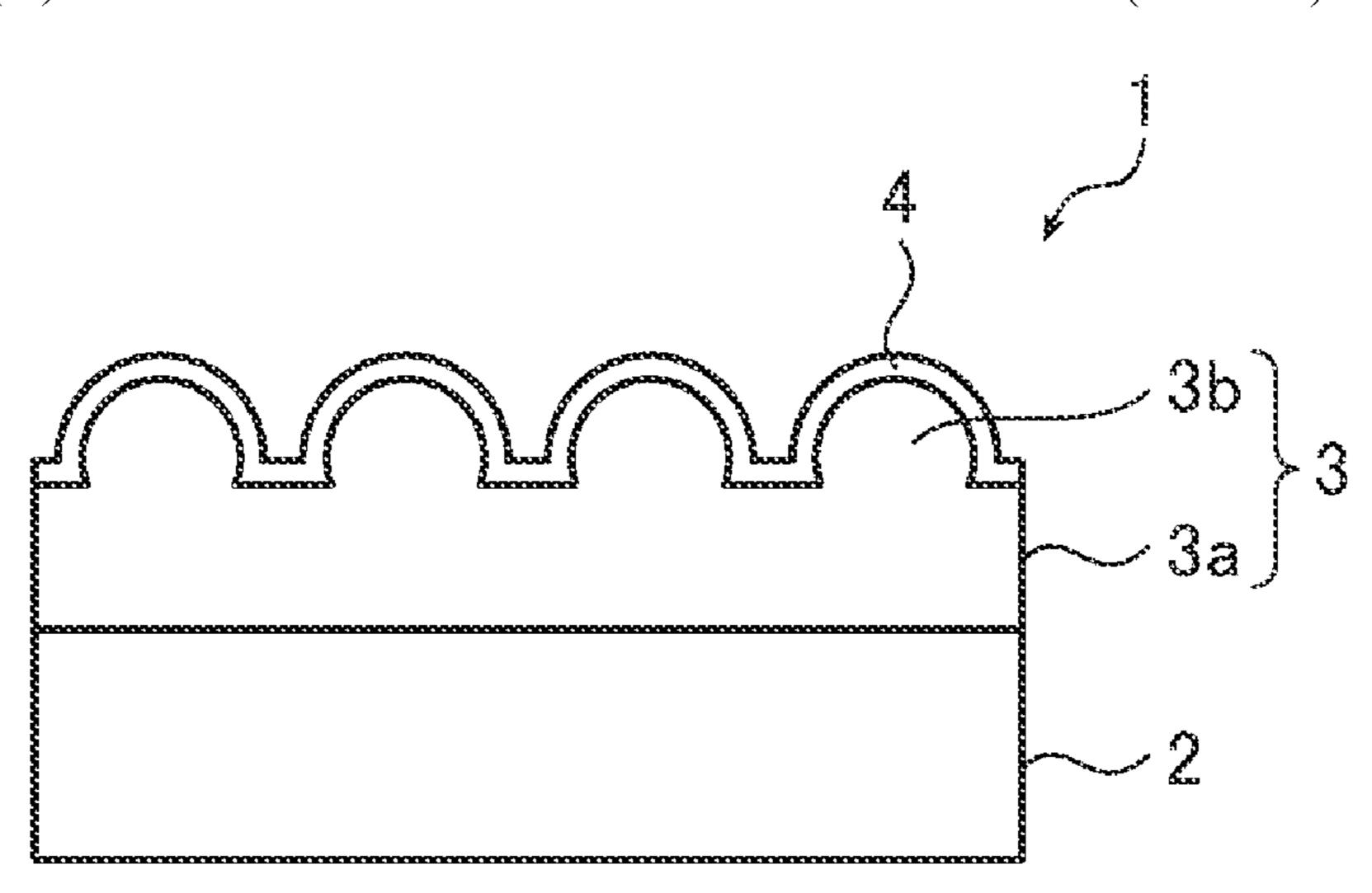
chromium oxide layer in terms of chromium is  $3-30 \text{ mg/m}^2$ . The chromium metal layer includes: a base part having a thickness of 7.0 nm or higher; and granular protrusions which are on the base part, have a maximum grain size of 100 nm or lower, and have a number density per unit area of at least  $200 \text{ per } \mu\text{m}^2$ .
