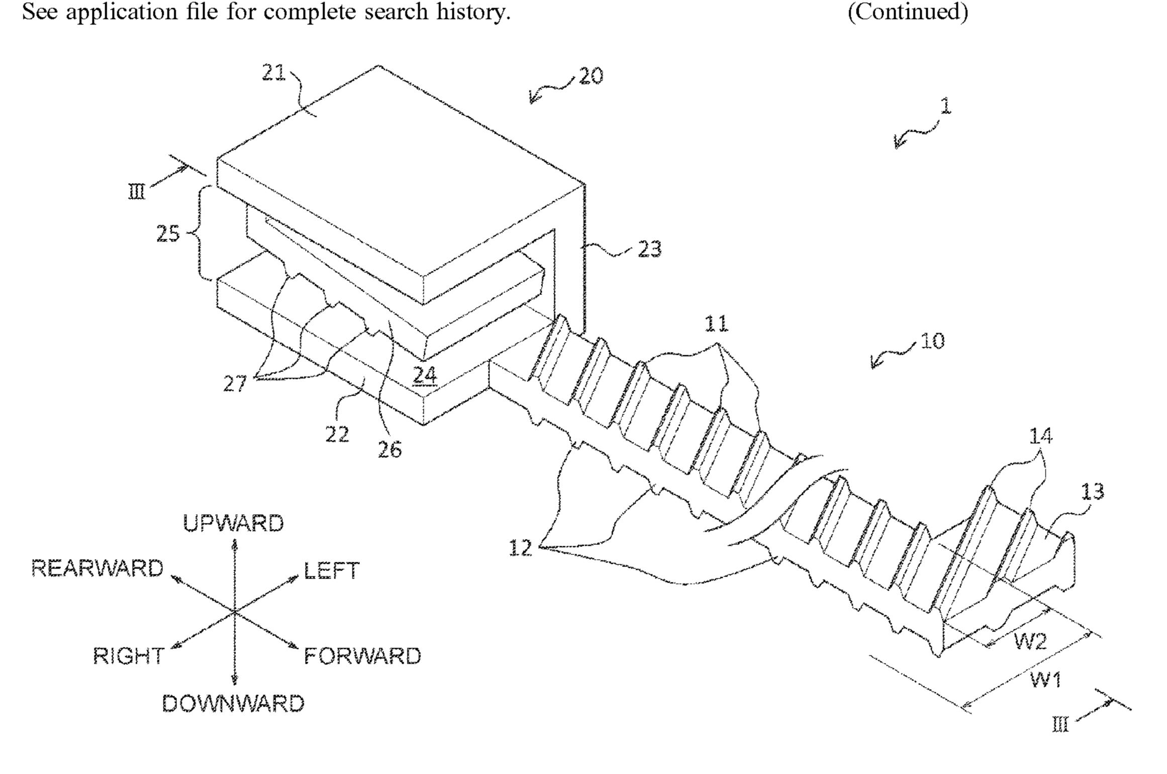
plurality of ratchet teeth and ratchet claws are inclined such that each of one end portions thereof on the one side in the width direction is on a downstream side of the extension direction as compared with each of the other end portions thereof on the other side in the width direction.
