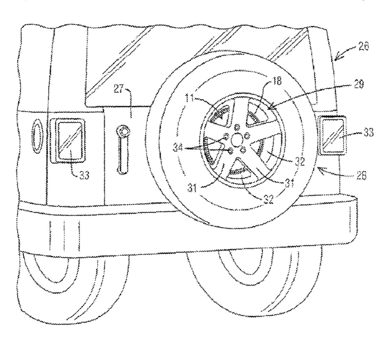
to be seen from behind as an indication that the vehicle is braking. A second portion of the ring of LEDs aligns behind the spokes and reflects off of the backs of the spokes to silhouette the rim against the glow of the reflected light.
