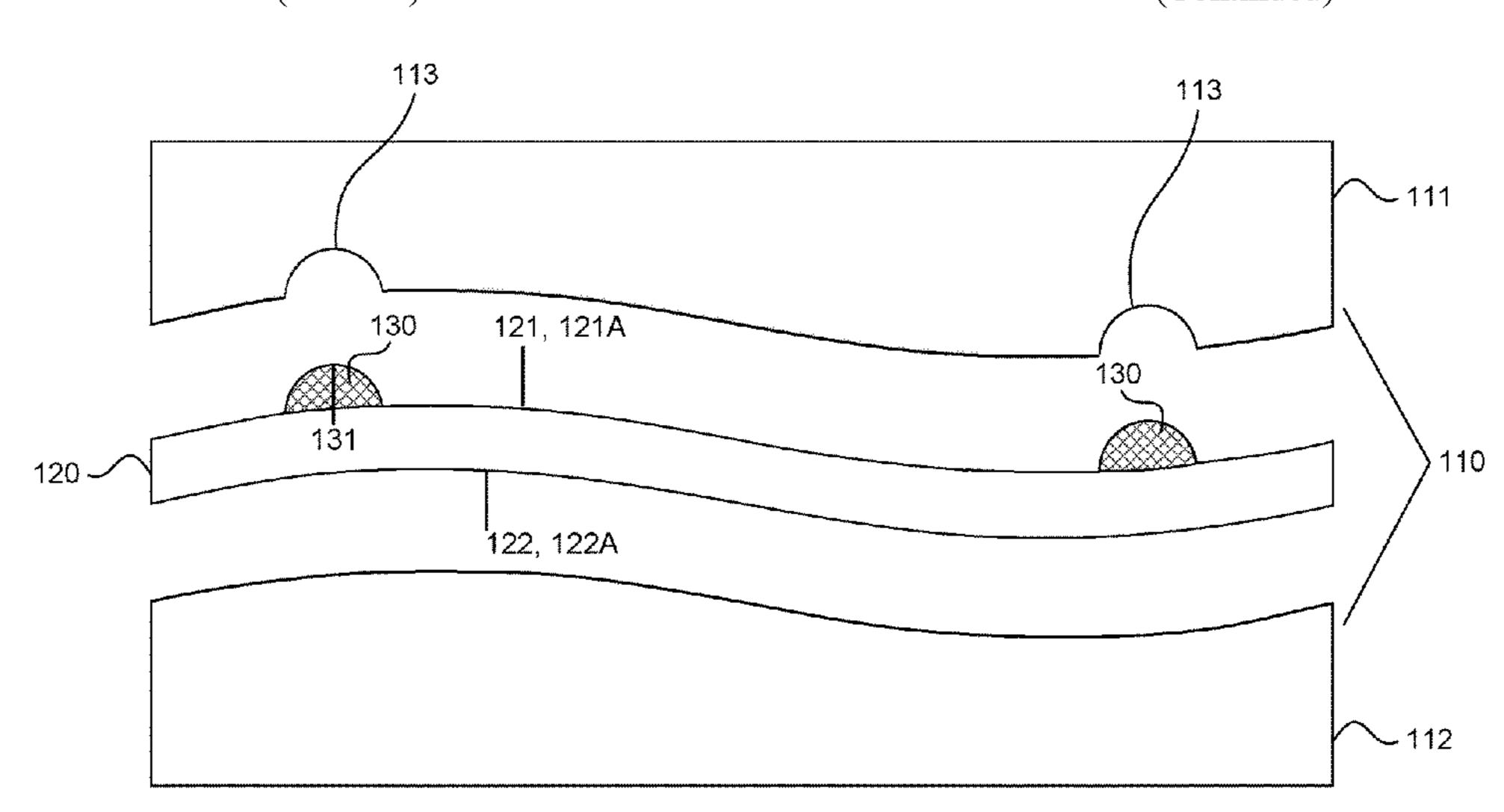
one another. The cold-formed glass substrate is attached to a rigid support structure having the curved shape. The cold-formed glass substrate includes an open region not in direct contact with the non-planar rigid support structure, and the open region has a curved shape maintained by the non-planar rigid support structure.
