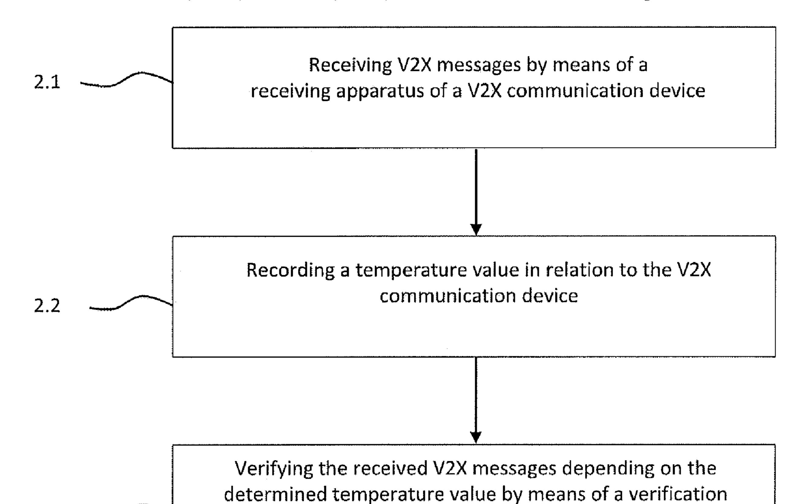
apparatus of the V2X communication device
