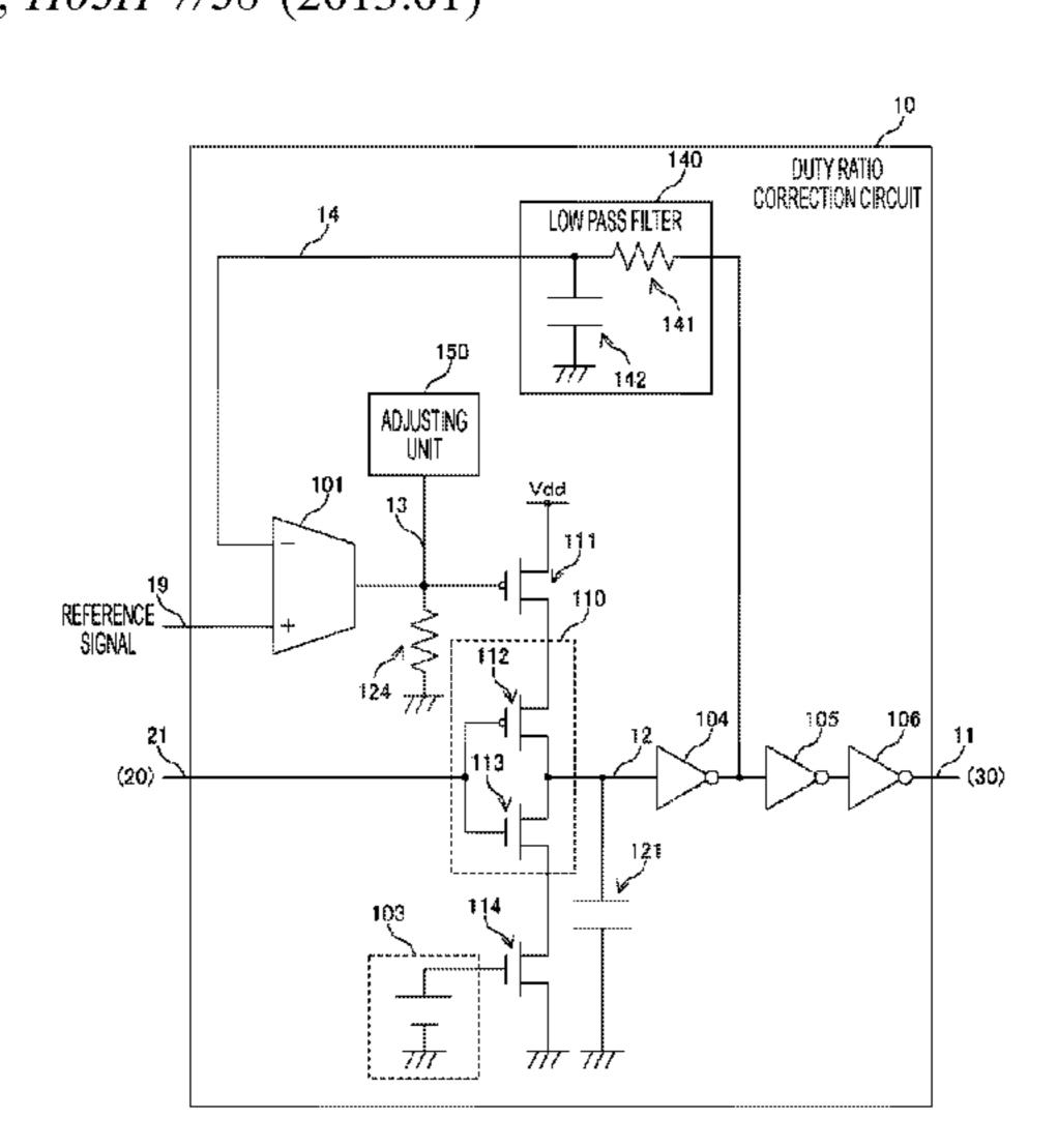
and a reference signal. The adjusting unit adjusts the control of the inverting buffer by the error amplifier.
