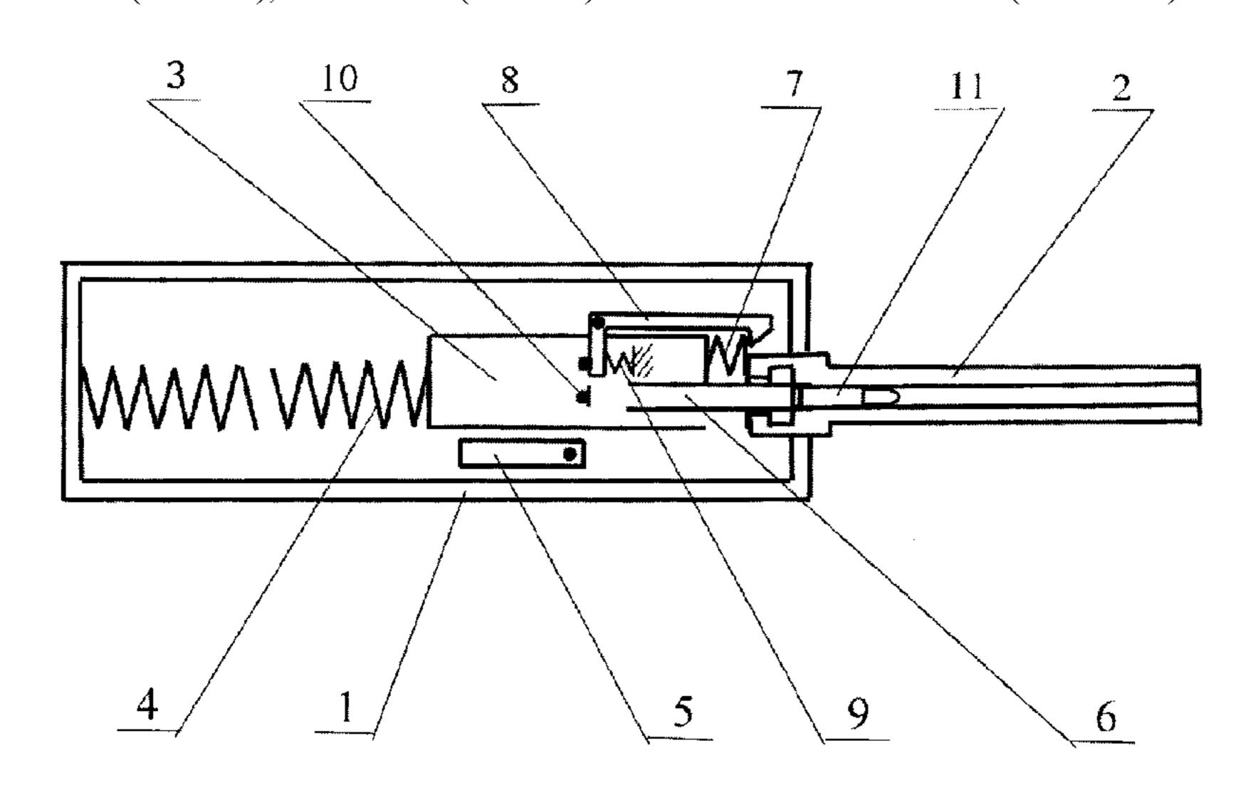
spring, and a lever for compressing and subsequently locking the bumper spring during the rearward movement of the bolt carrier in the case of manual reloading, wherein said lever can be combined with a recharging handle. The technical result provided by the above combination of features is the creation of a firearm having an inertial automatic loading system that functions reliably and consistently due to the increased reloading system working speeds and increased recovery of recoil energy.
