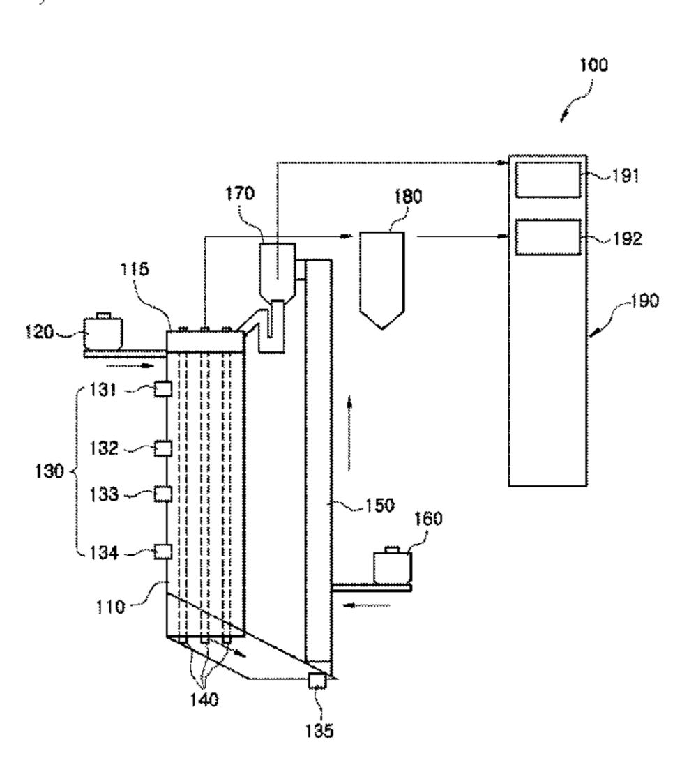
and oxidizer are injected, a riser section connected to the boiler section so that the fuel and fluid sand supplied from the boiler section are introduced from the bottom of the riser section and flow up, and a relay section provided on the boiler section to supply the fluid sand having passed through the riser section to the boiler section, wherein the fuel is injected from the top of the boiler section and burned while flowing down therein.
