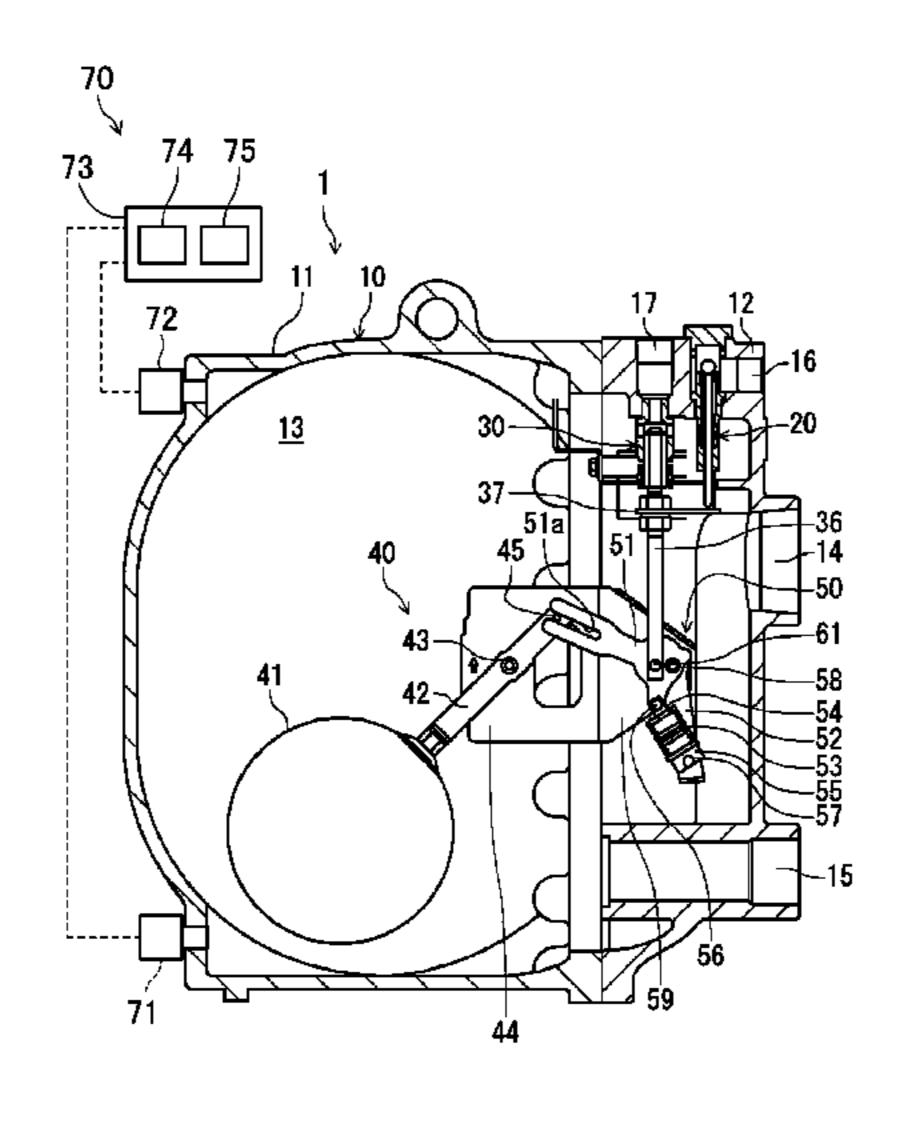
tion device includes a first pressure sensor arranged to communicate with a lower portion of the reservoir space to detect a pressure of a liquid layer in the reservoir space, and a deterioration determination unit that determines a degree of deterioration of the valve operating mechanism based on a change in the pressure detected by the first pressure sensor.
