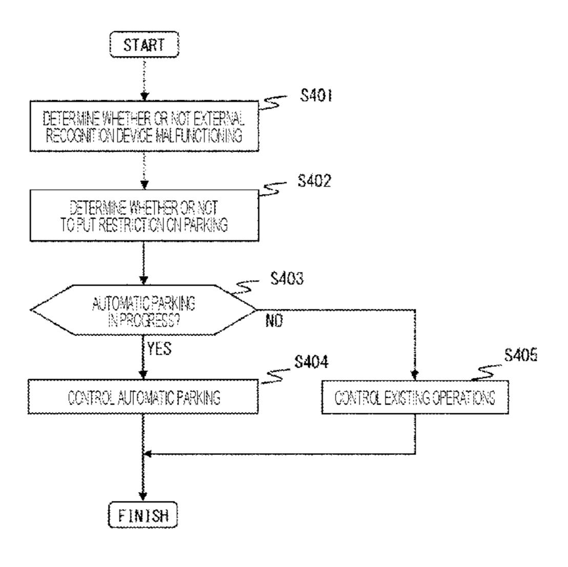
with the malfunction of the camera, and for restricting the path in accordance with the malfunction of the sonar. Next, in processing S403, a determination is made whether or not the automatic parking is in progress. When the automatic parking is in progress, the process proceeds to processing S404 where vehicle speed control or the like is performed for the automatic parking in accordance with the malfunction of the external recognition device.
