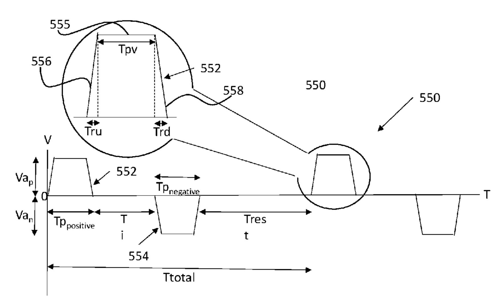
the positive voltage pulse attains at least 80% of the time-averaged voltage amplitude, within a time (T80) of 70-150 nanoseconds; (2) the positive voltage pulse increases by at least 20 Volts, within 70 nanoseconds.
