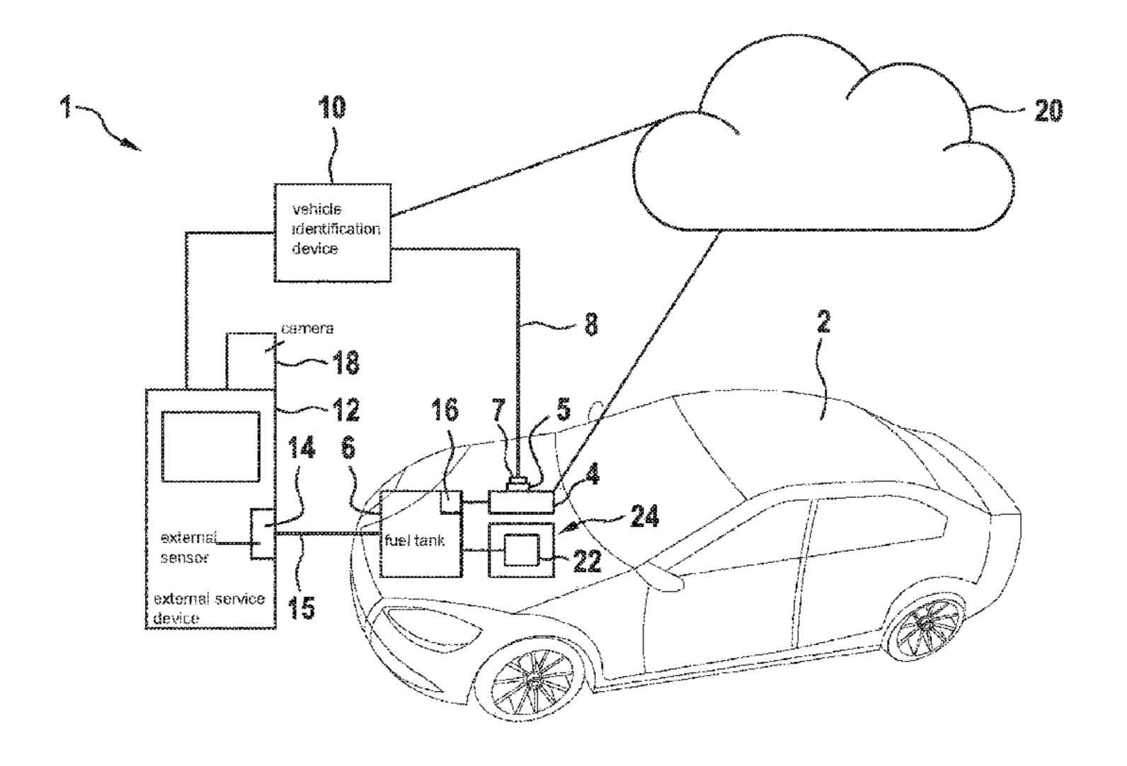
cation device. The external sensor detects the physical interaction and transmits a corresponding external detection value to the vehicle identification device; and the vehicle identification device compares the vehicle detection value and the external detection value with one another and confirms the identity of the vehicle if the two detection values coincide with one another within a predefined tolerance.
