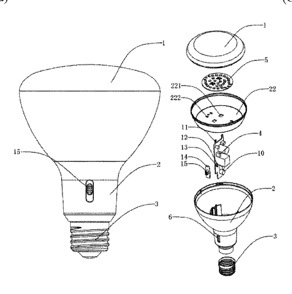
color temperature, the timing or the light intensity of the LED light by multiple positions of the shift switch.
