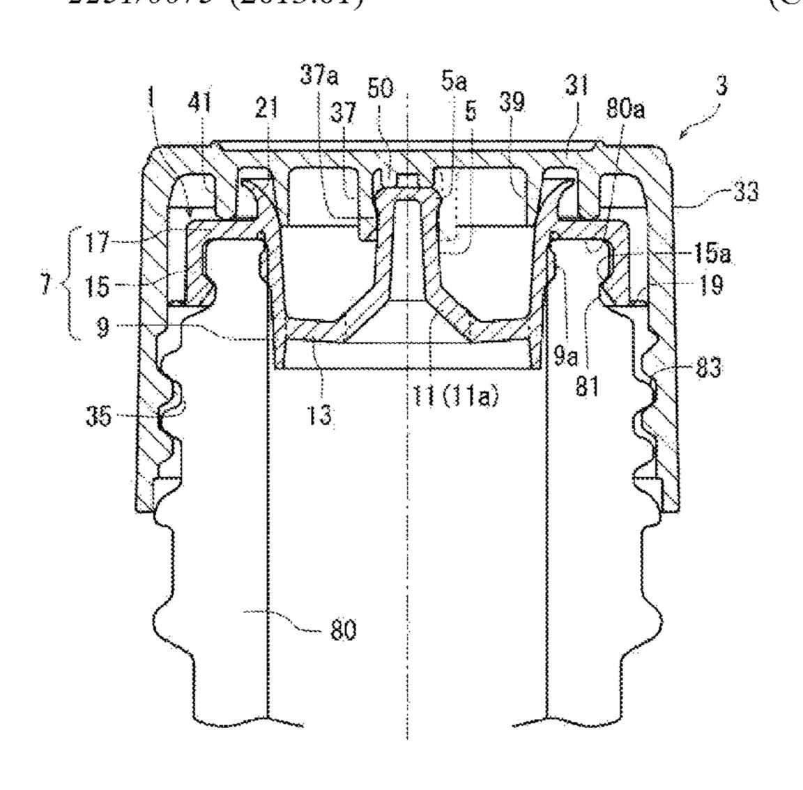
engaging with the circumferential protuberance 5a that temporary engages with the upper lid engaging cylinder; and a sound-suppressing protrusion 50 is provided in a region surrounded by the engaging pieces 37.
