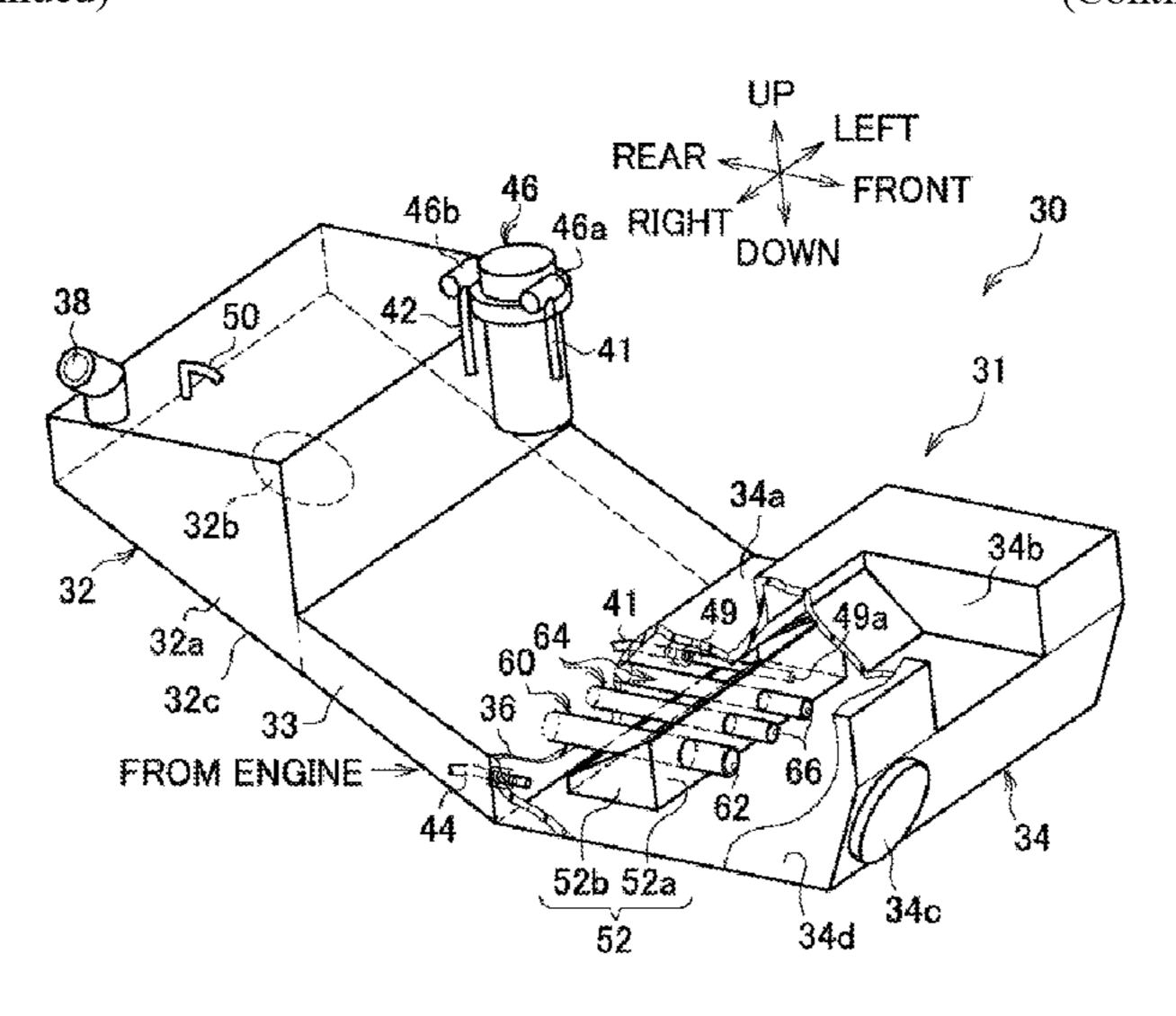
second end having a hollow tube opening (62) extending and opened toward the center of the vehicle body inside the second storage tank, wherein the hollow tube opening of the hollow tube member is located on the central side of the vehicle body with respect to the discharge opening of the discharge member.
