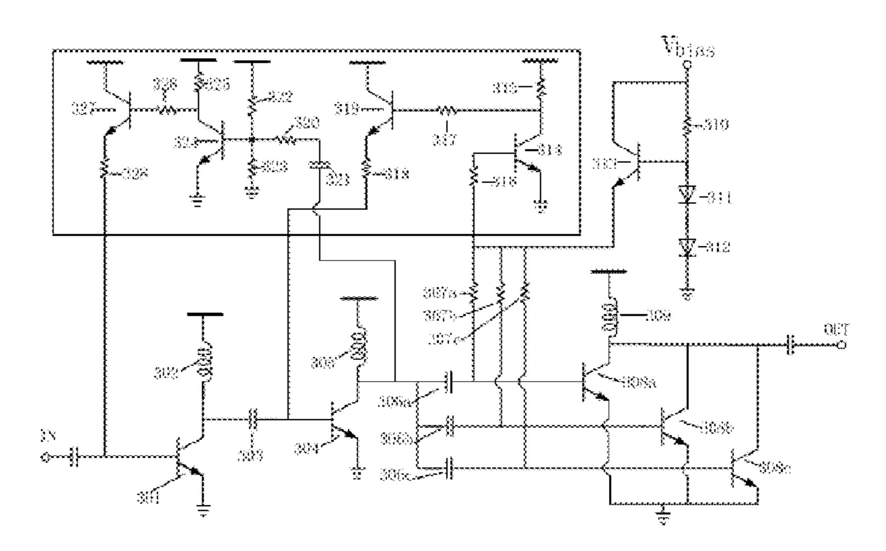
power of the current stage of amplifier circuit, a control voltage varying inversely with the output power, so that the power detection feedback circuit outputs current varying positively with the control voltage.
