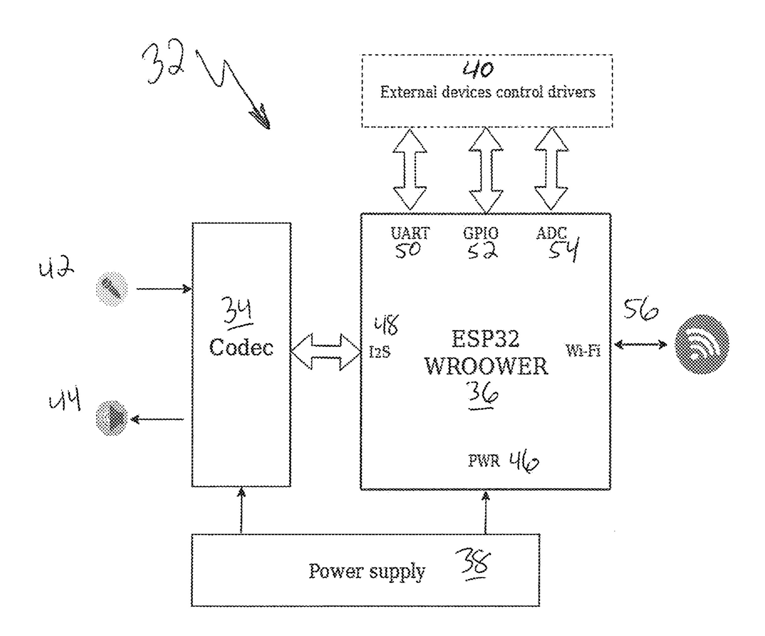
FIG. 3. VOI Bridge Components Diagram
