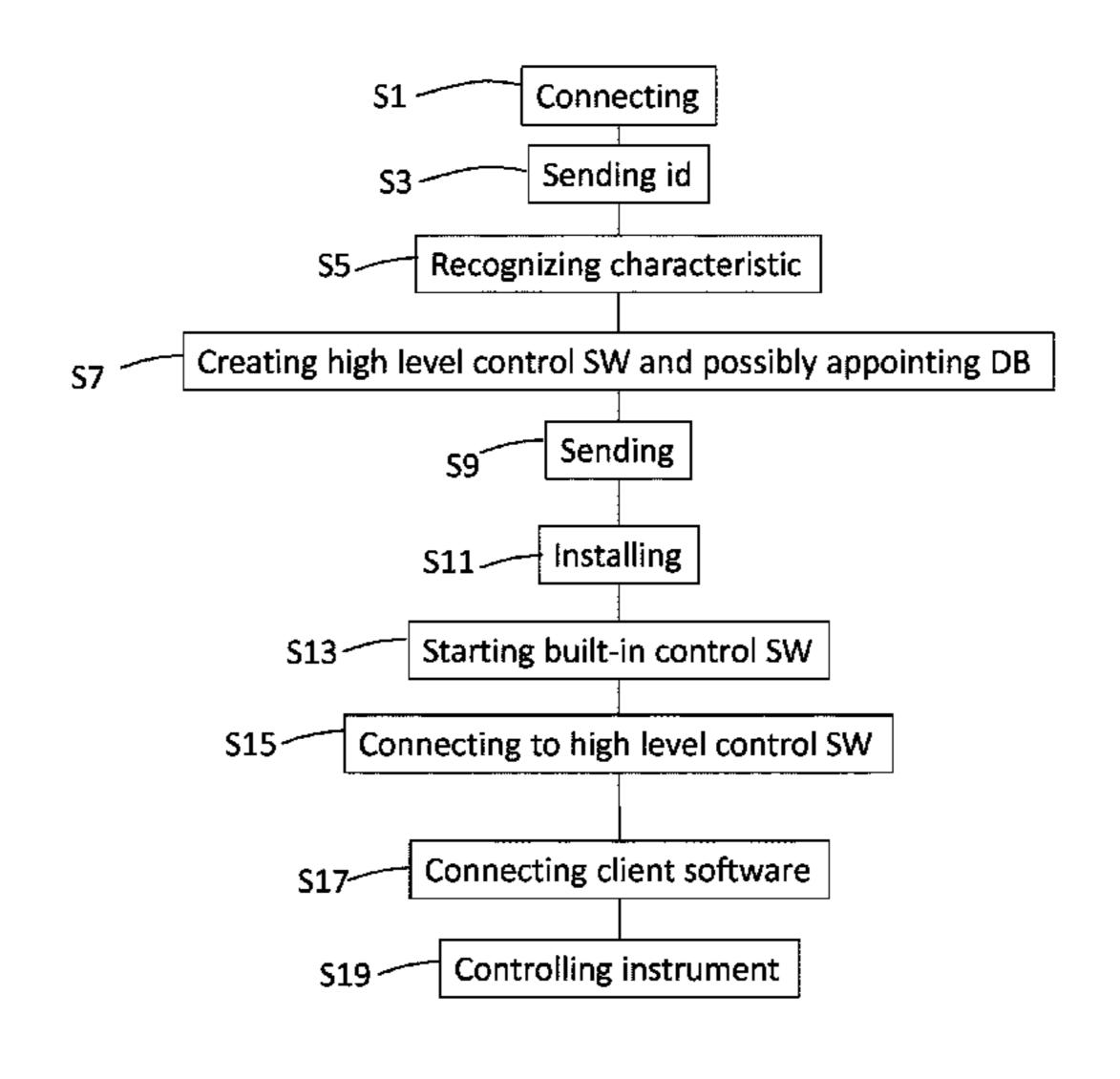
control software dedicated for the instrument via the first, or a second communication interface (16), said built-in control software using the low level control software to monitor and control the instrument.
