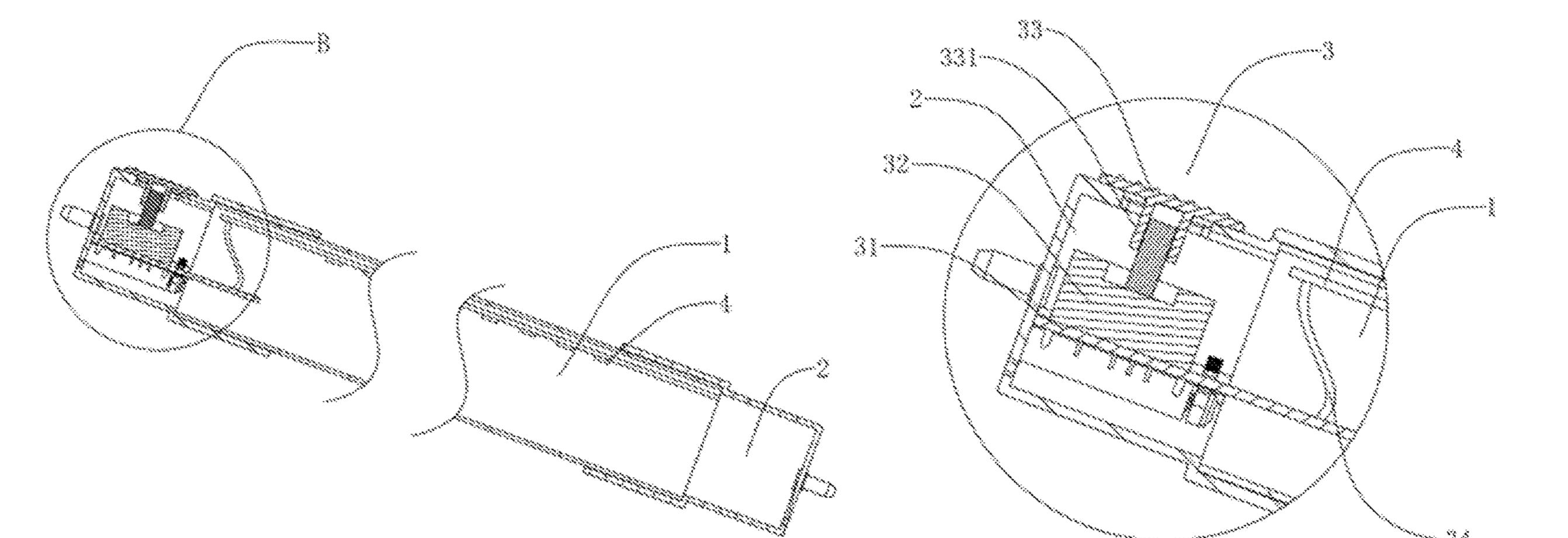
LED tube light body further includes at least one color adjustment switch fixed on the respective terminal. The color adjustment switch is configured to control the on and off of different color temperatures of the LED light strip.
