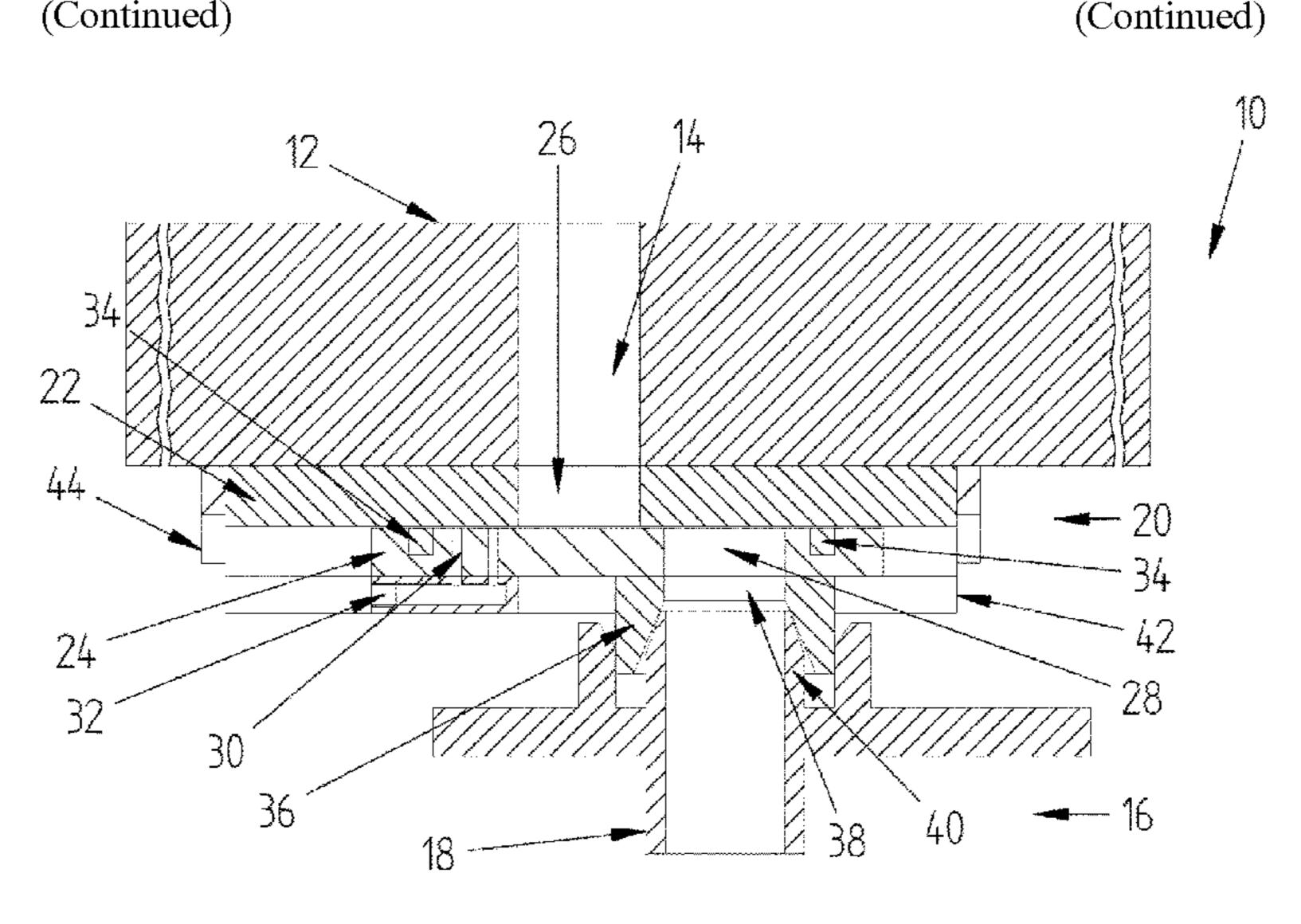
position, the second opening is arranged to align with the opening of the base plate, at least to the greatest possible extent; and in the closure position, the gate valve plate closes off the opening of the base plate.
