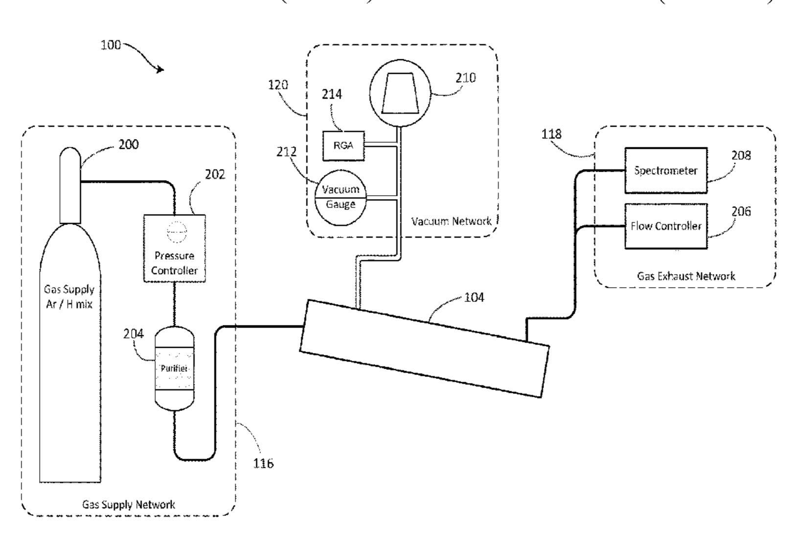
the gas exhaust tube. A vacuum network is coupled in flow communication with one end of the vacuum port. A method and apparatus for purifying target material also are described.
