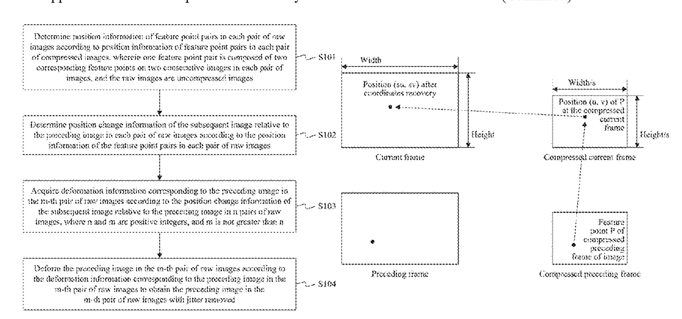
deforming the preceding image in the m-th pair of raw images according to the deformation information corresponding to the preceding image in the m-th pair of raw images for removing jitter in the preceding image in the m-th pair of raw images.
