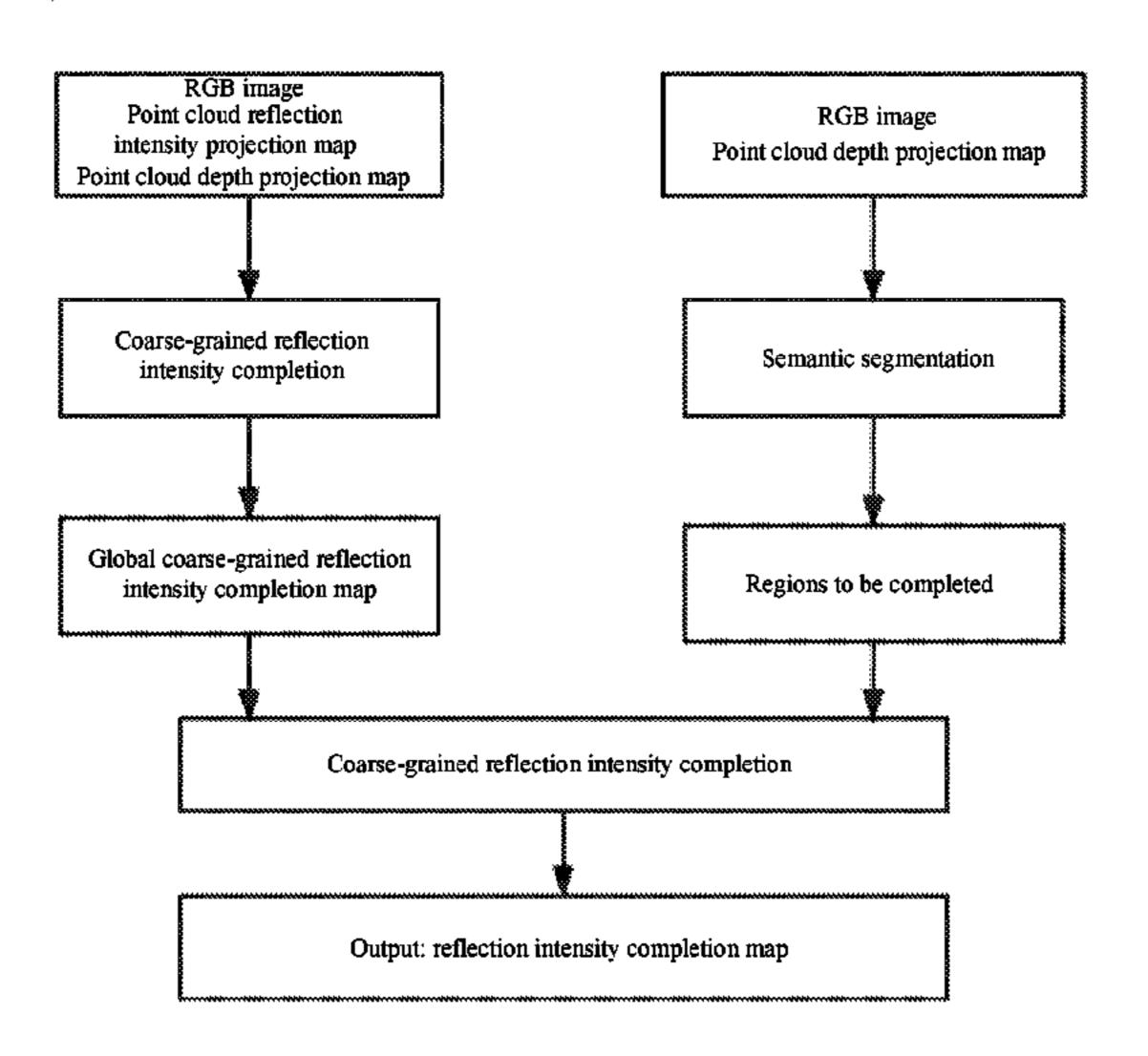
single-channel depth projection map to obtain a two-dimensional coarse-grained reflectance intensity projection map.
