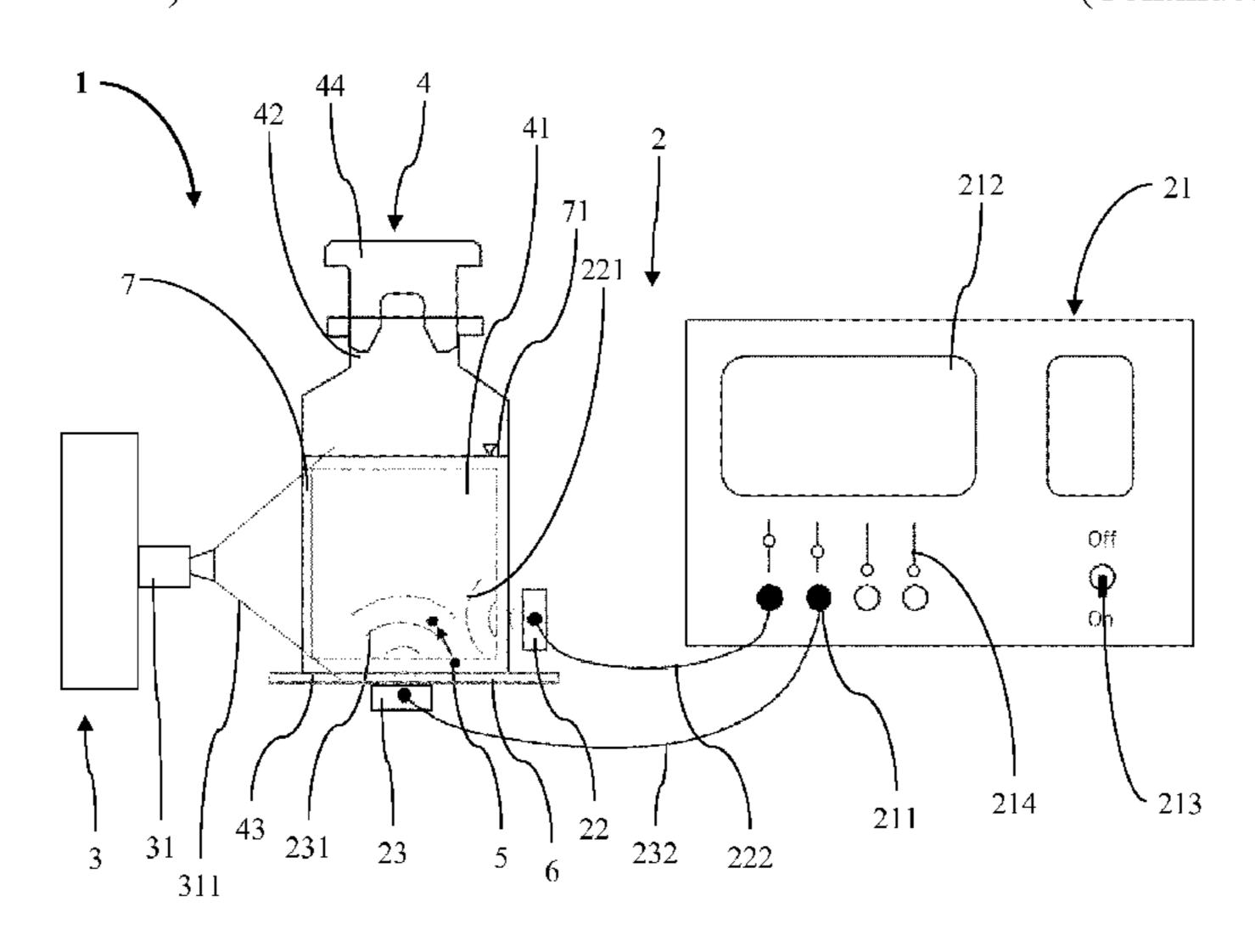
acoustic wave. The seat is adapted to position the container adjacent to the transducer for inspecting a liquid inside a container with respect to the existence of particles. The inspection device allows for an accurate and gentle inspection of the liquid filled in the container and for detecting particles in the liquid.
