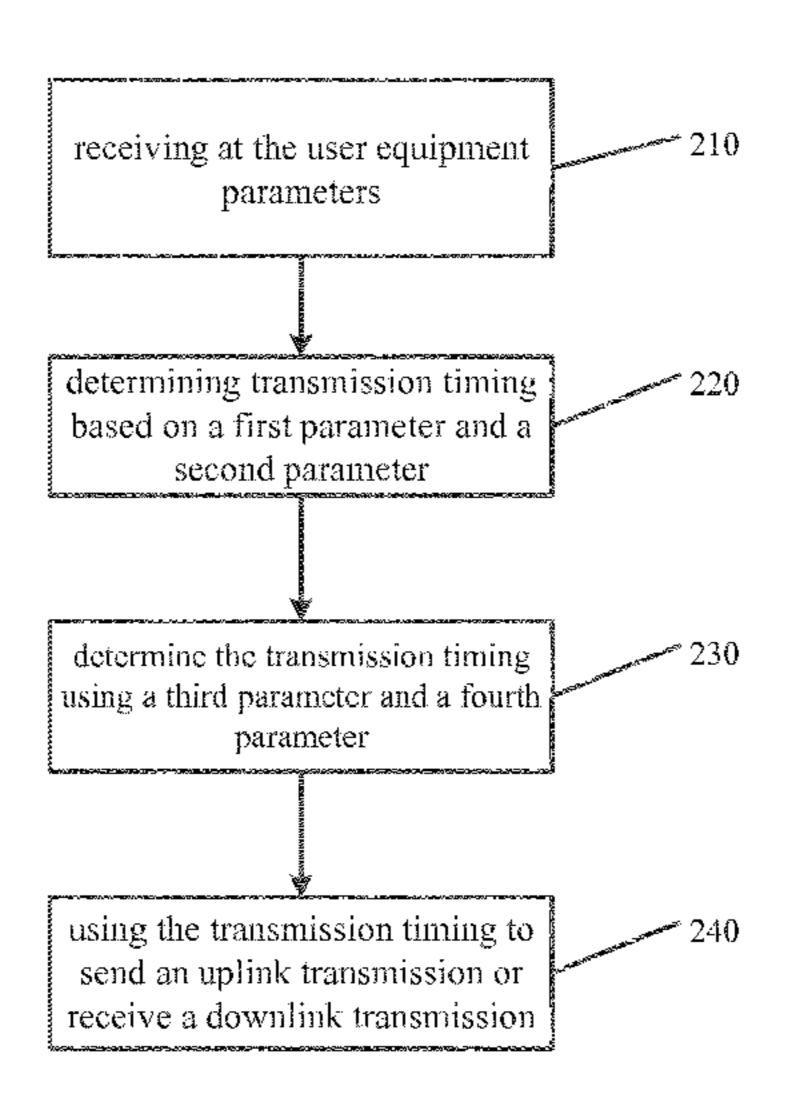
method may also include using the transmission timing to at least one of send an uplink transmission or receive a downlink transmission.
