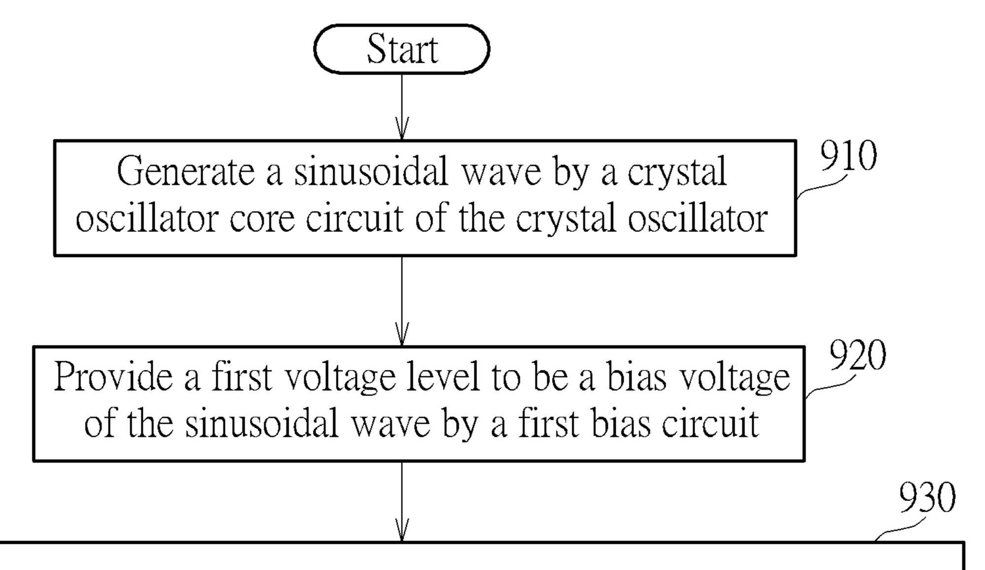
Reset the bias voltage of the sinusoidal wave by a phase noise reduction circuit of the crystal oscillator in response to a voltage level of the sinusoidal wave exceeding a specific voltage range
