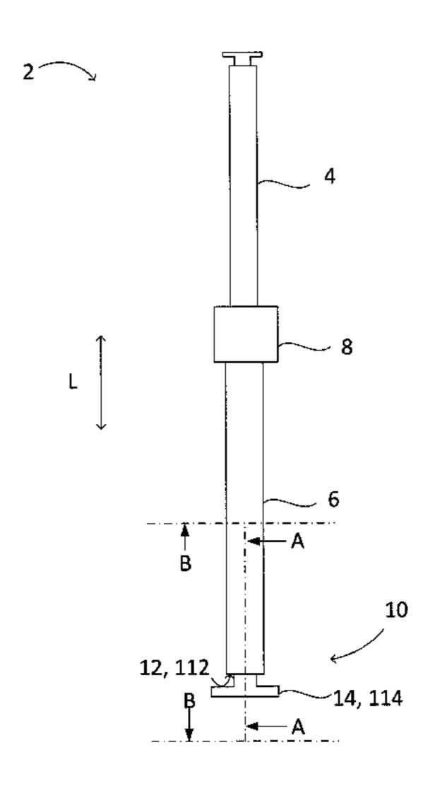
spring. The lever is arranged in a second position in a stressed condition of the spring. By moving the lever from the first position to the second position, and vice versa, resiliently affect the surface support element (14; 114) in a direction to and from the open end (10) of the support post (2). The surface support element is arranged to be installed on a floor, and the lever is a pedal.
