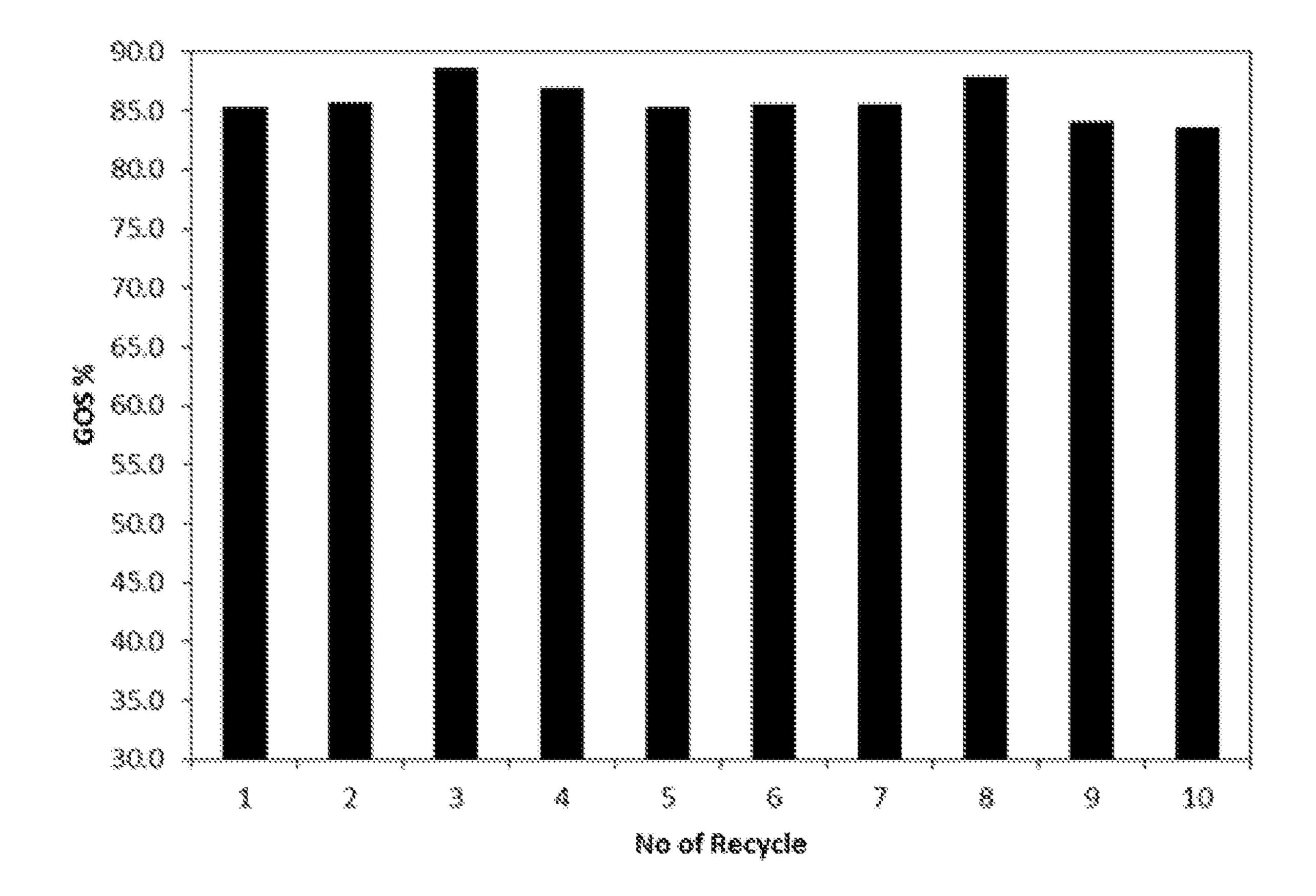
Figure 2: Galacto-oligosaccharides yield data of 10 cycles using the process of the present disclosure
