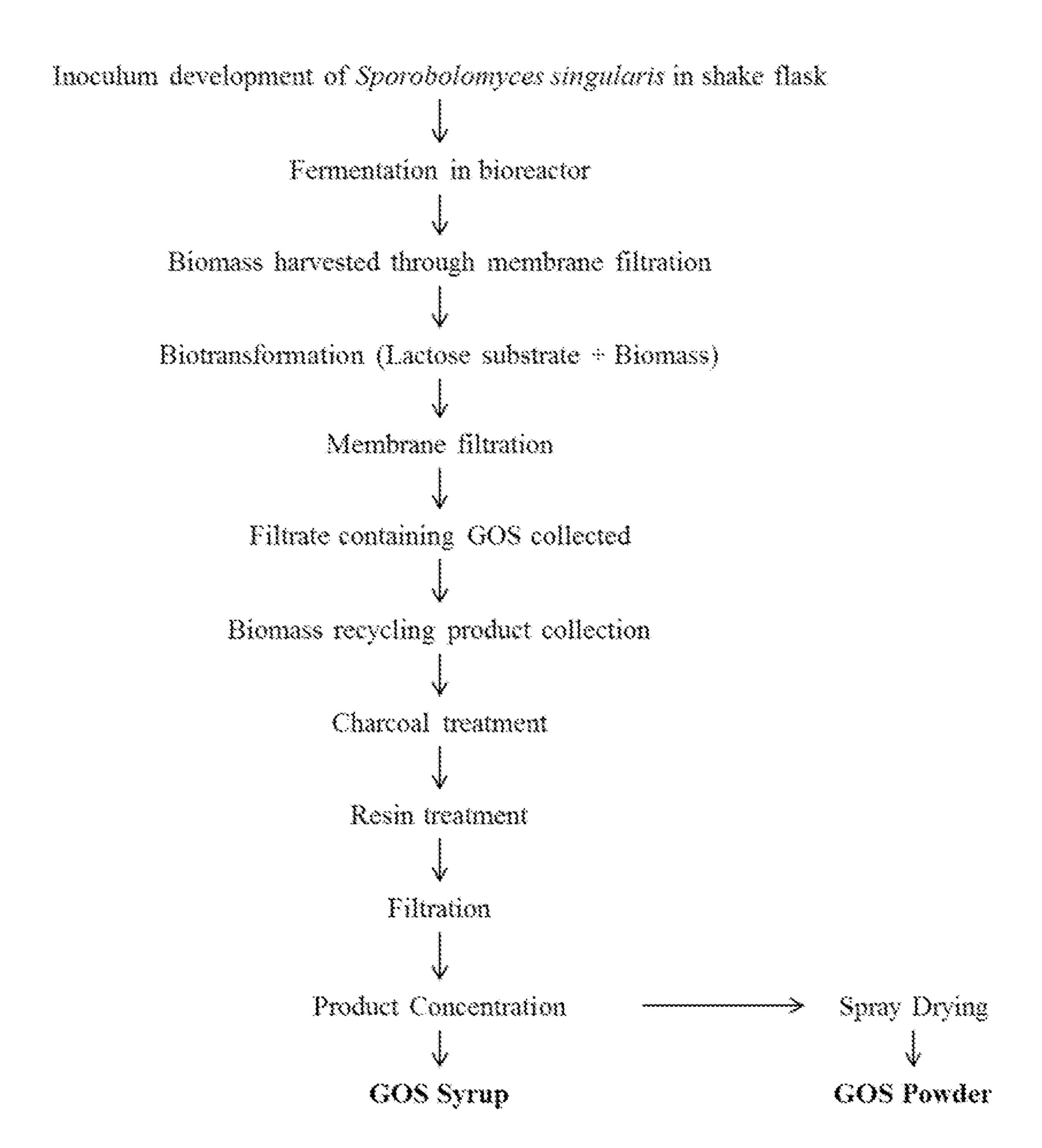
Figure 1: Process flow diagram of producing galacto-oligosaccharides in accordance with an embodiment of the present disclosure
