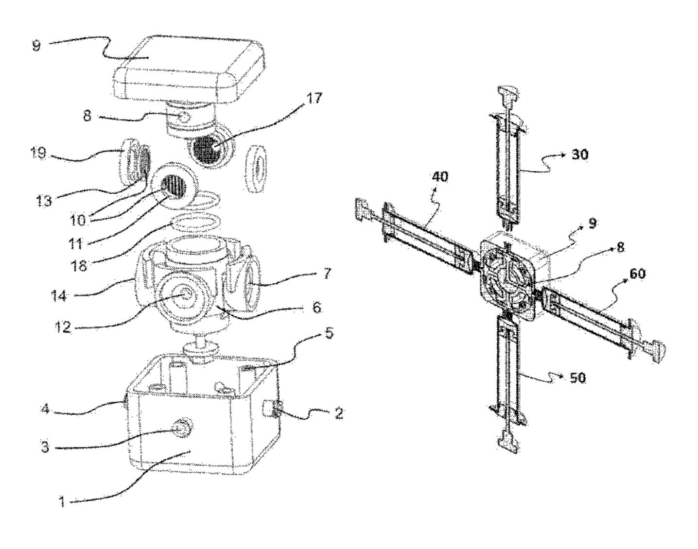
movement, at least one cover (10) which enables the said movement of the passage (8) and covers the top of the reservoir (1), a second inlet (12) which comprises a first splitting element (11) that is obtained by alignment of a multiple of cutting elements (10), and a third inlet (14) which comprises at least one second splitting element (13) which enables the adipose tissue split when it enters to and exits from the injector and is obtained by alignment of a multiple of cutting elements (10).
