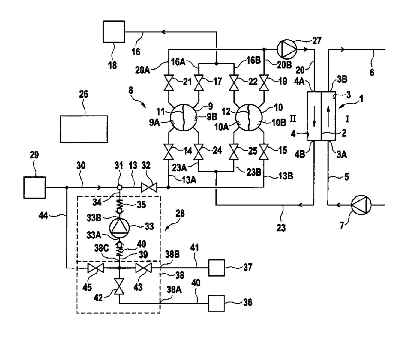
using just one single metering pump. This is advantageous in that the metering pump is a relatively expensive component of the mixer circuit. In practice, the design is simpler and compact and the maintenance costs are reduced.
