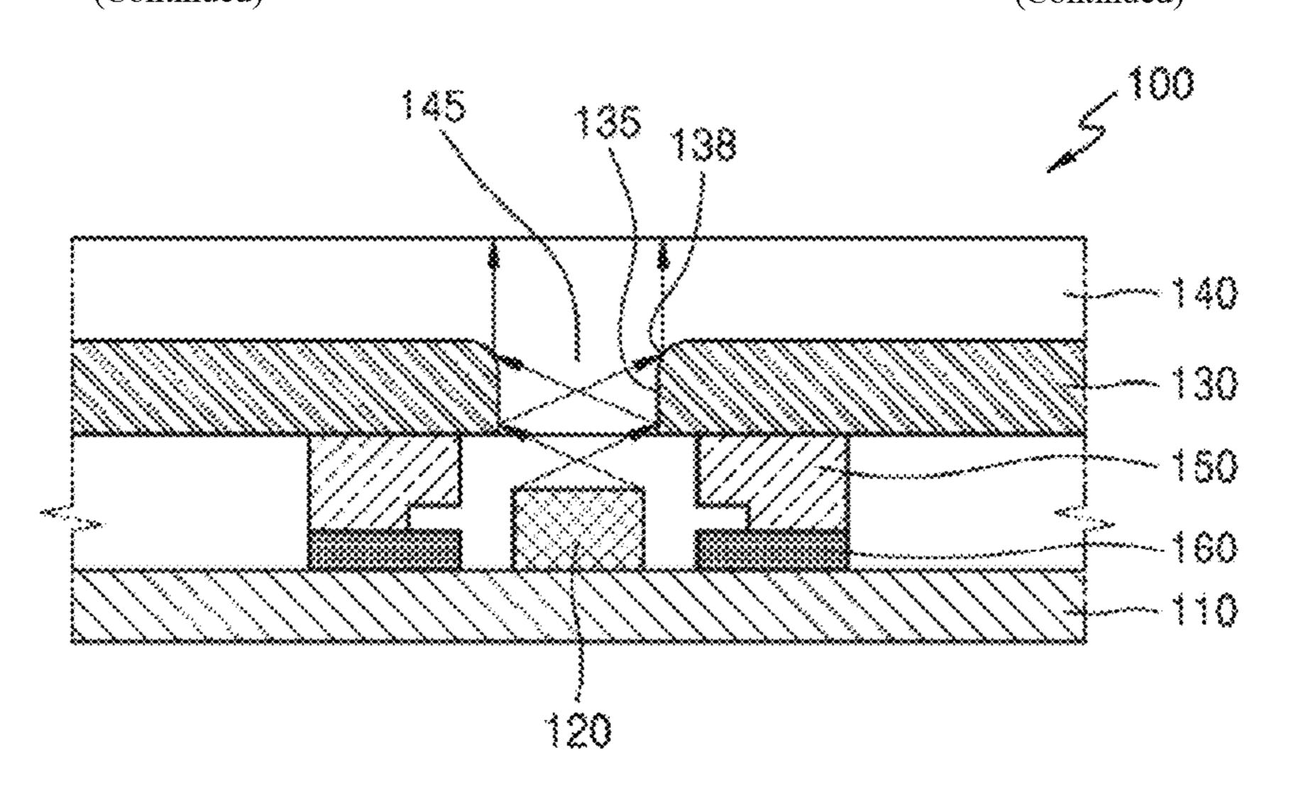
and widened in the direction away from the light emitting portion such that spread of light that passed through the opening is prevented.
