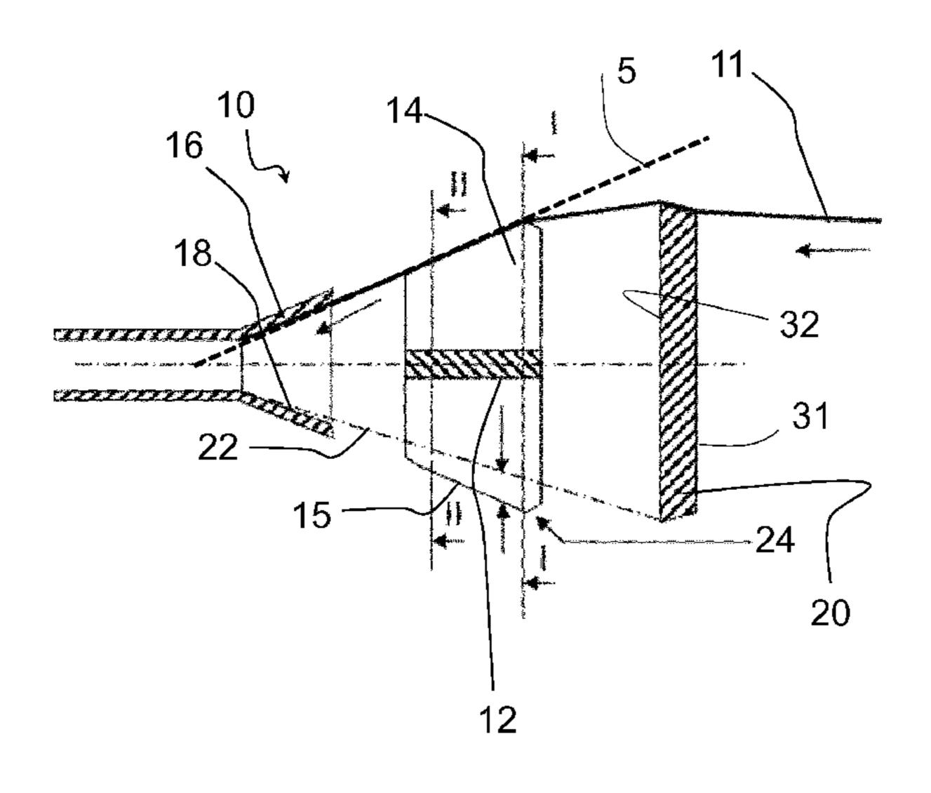
can partly fold within spaces defined between the spaced apart walls; and inserting the sheet of material into a funnel (16) to form a rod. The present invention also relates to an apparatus (10) to fold a sheet of material into a rod for an aerosol generating article.
