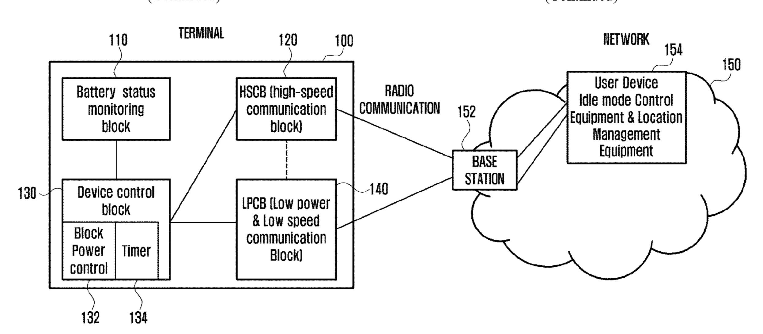
in a mobile communication system according to an embodiment of the present specification comprises the steps of: acquiring cell-related information corresponding to a first communication mode; acquiring cell-related information corresponding to a second communication mode; receiving a first message through the second communication mode; and transmitting a request message corresponding to the first communication mode on the basis of the first message.
