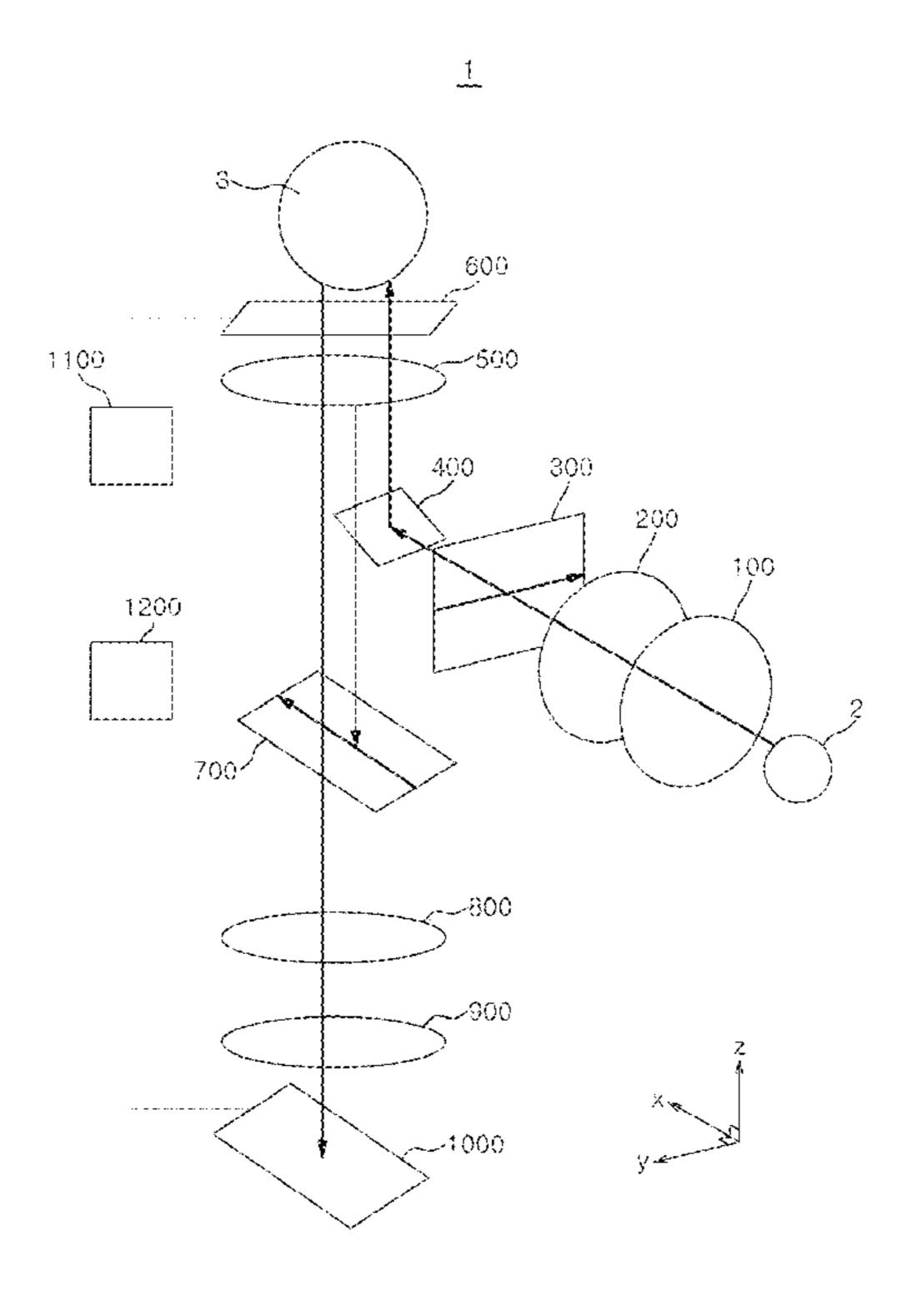
polarizer allows second polarized light oscillating in a second direction to proceed toward the detection unit when the emission light reaches the second polarizer.
