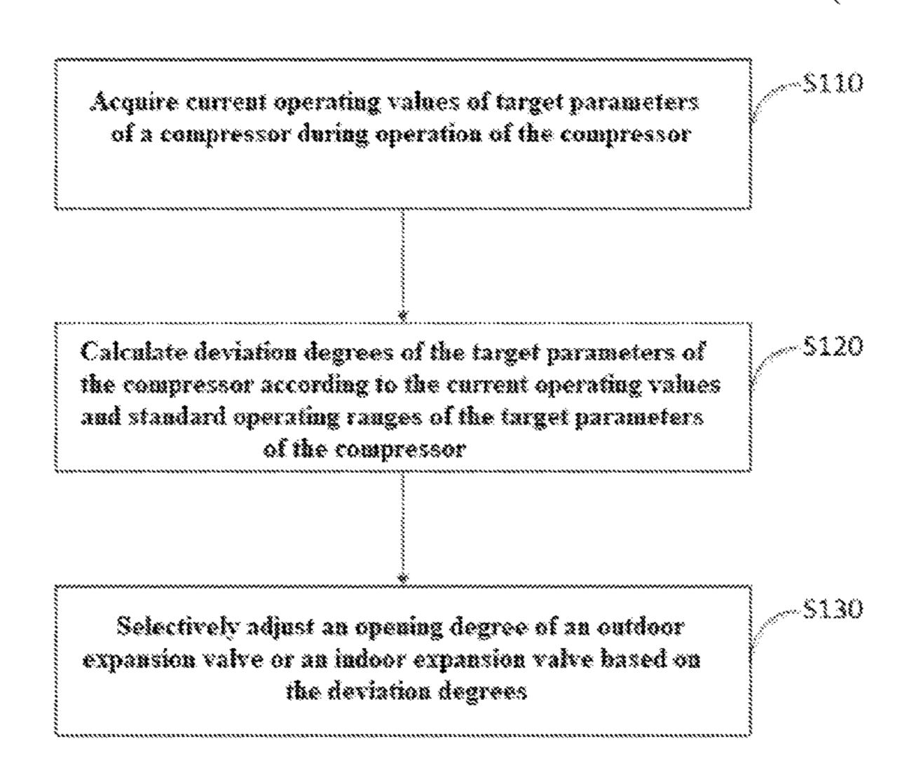
of the indoor expansion valve or the outdoor expansion valve is adjusted in real time according to parameters of the compressor.
