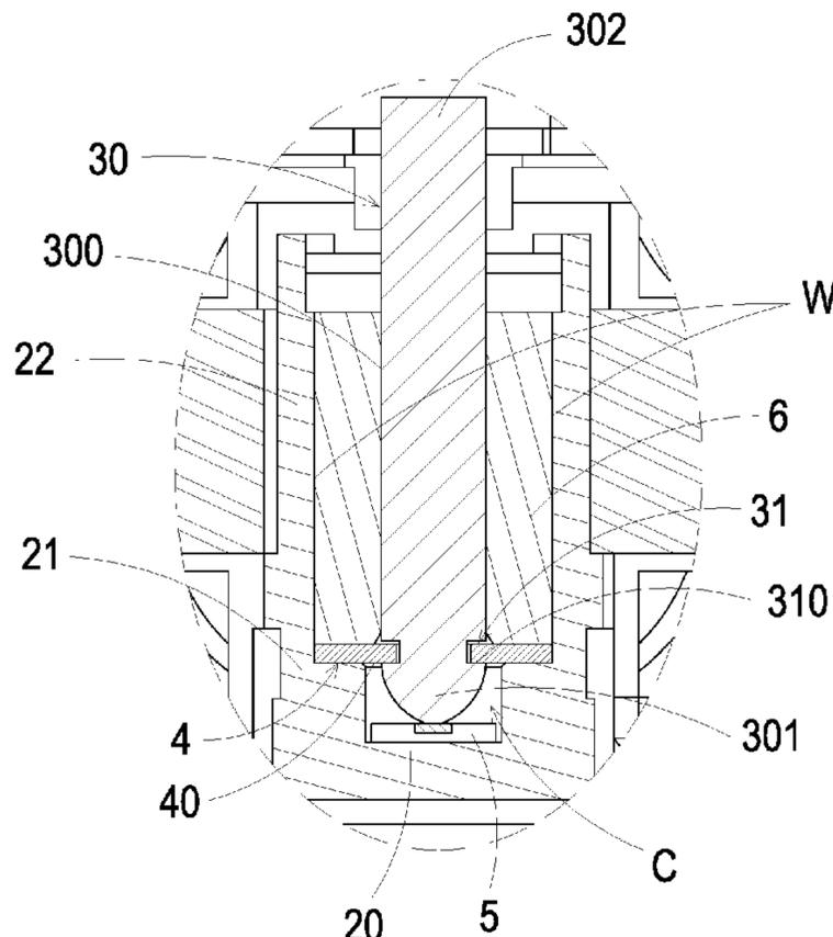
limiting element is disposed on the sleeve and extended from the side wall toward the rotating shaft, and the position limiting element has a bottom surface. The bottom surface faces toward the bottom portion, and the bottom surface is interfered with the surface, thereby eliminating the gap between the bottom surface and the surface. Therefore, noise of the up and down vibration is avoided from generating.
